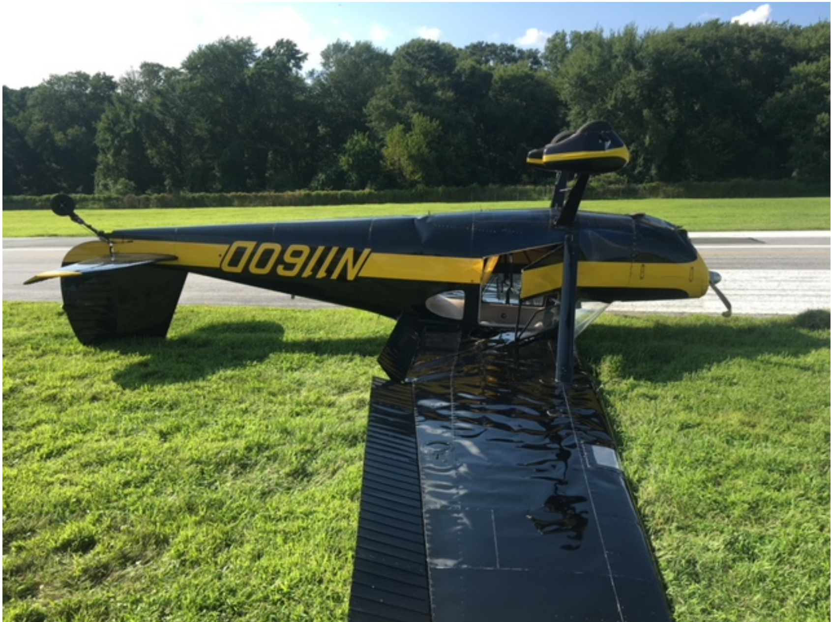
Photo 1 – View of damage to the right wing, vertical stabilizer and rudder (Courtesy of FAA)
