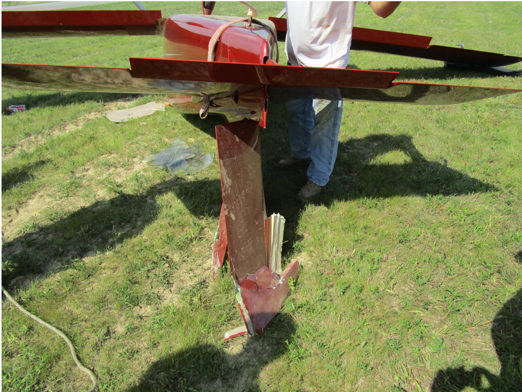
Photo 1 – View of damaged empennage from rear (Photo courtesy of the FAA)
