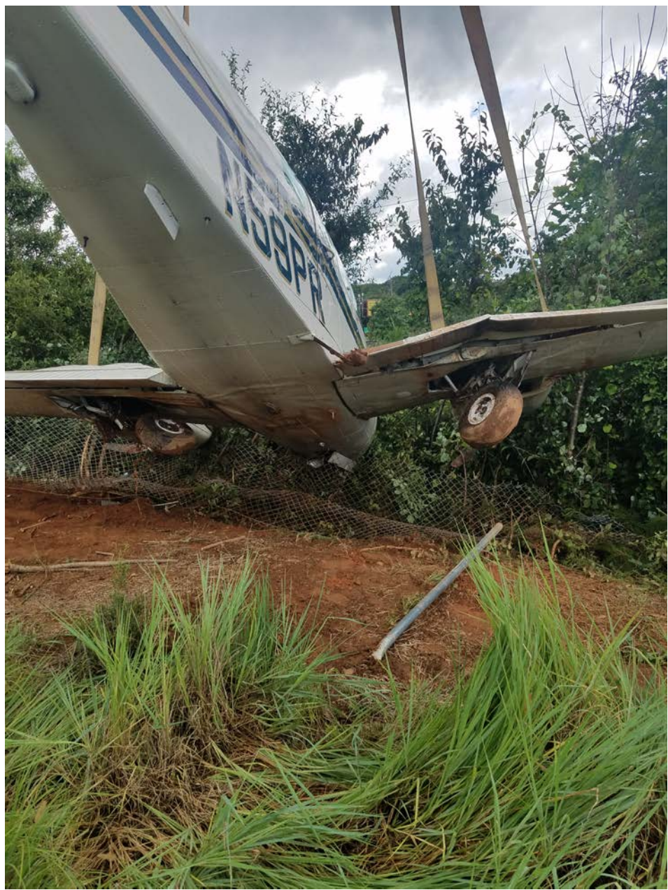
Photo 1 – View of damage to both wings and the fuselage (Courtesy of FAA)
