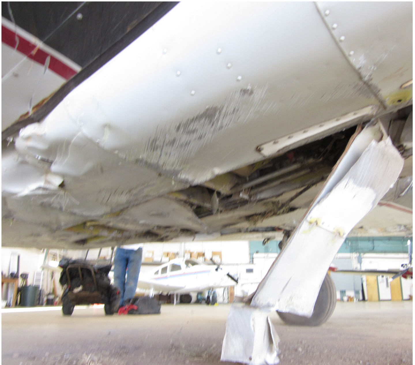
Photo 1 – View of damage to the longerons (Courtesy of FAA)
