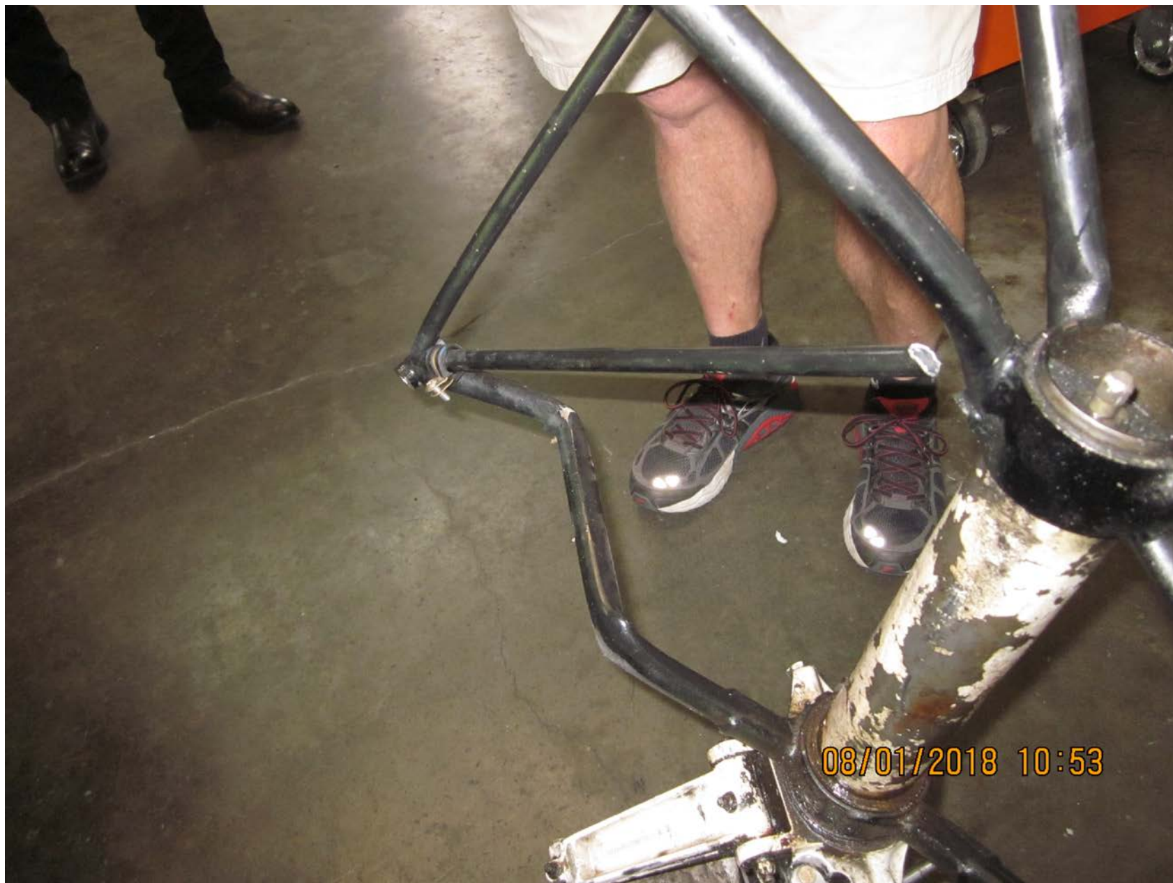
Photo 1 – View of the damaged engine mounts (Courtesy of FAA)
