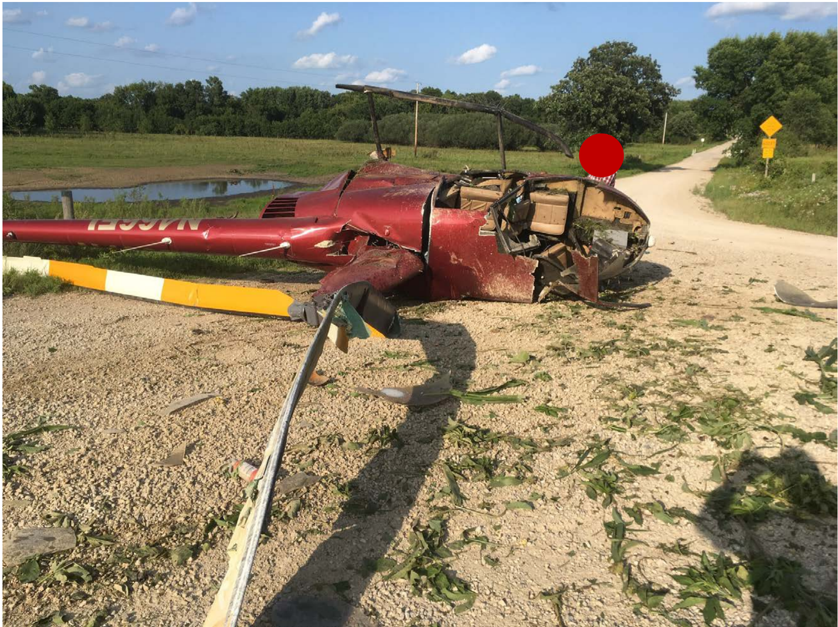
Photo 1 – View of damage to the fuselage and main rotor blades (courtesy of the FAA)
