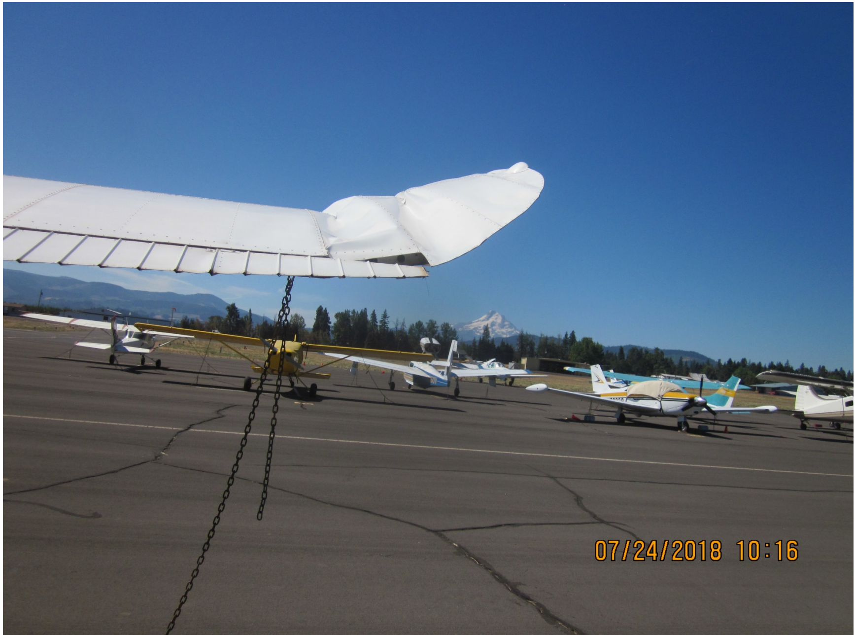
Photo 2 – View of damaged right wing (Photo courtesy of the FAA)
