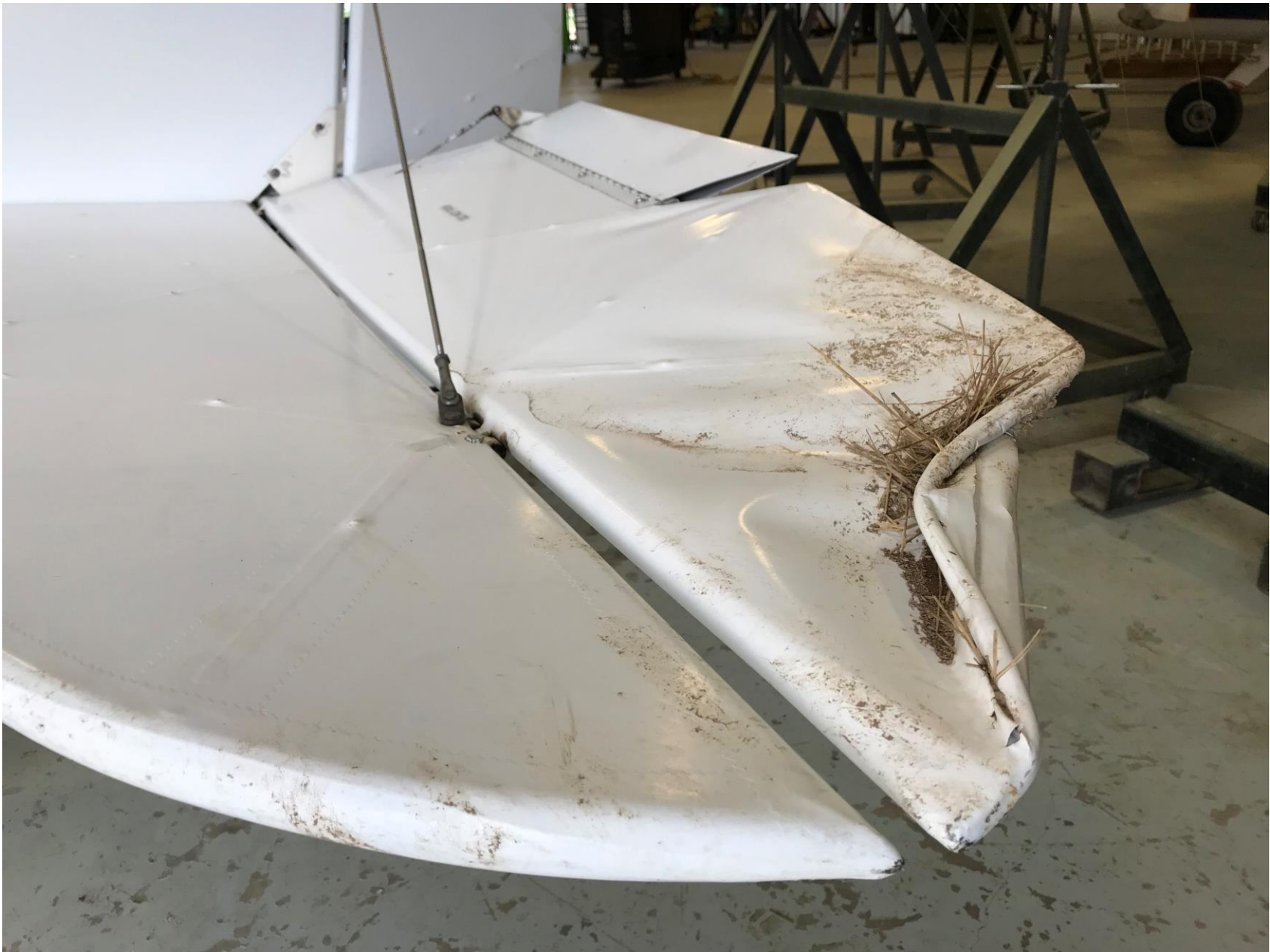
Photo 2 – View of damaged elevator (Photo courtesy of the FAA)
