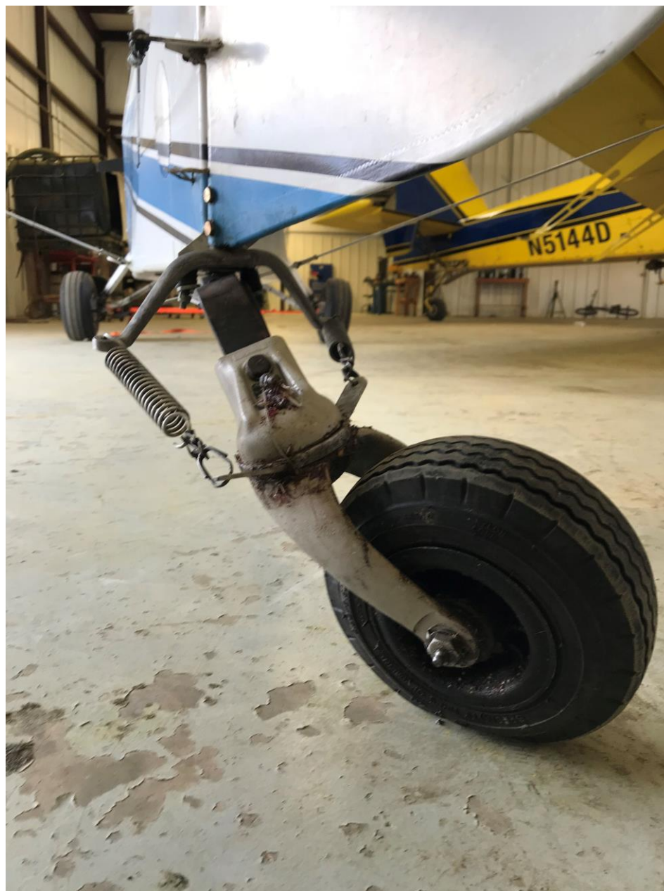
Photo 3 – View of damaged tailwheel (Photo courtesy of the FAA)
