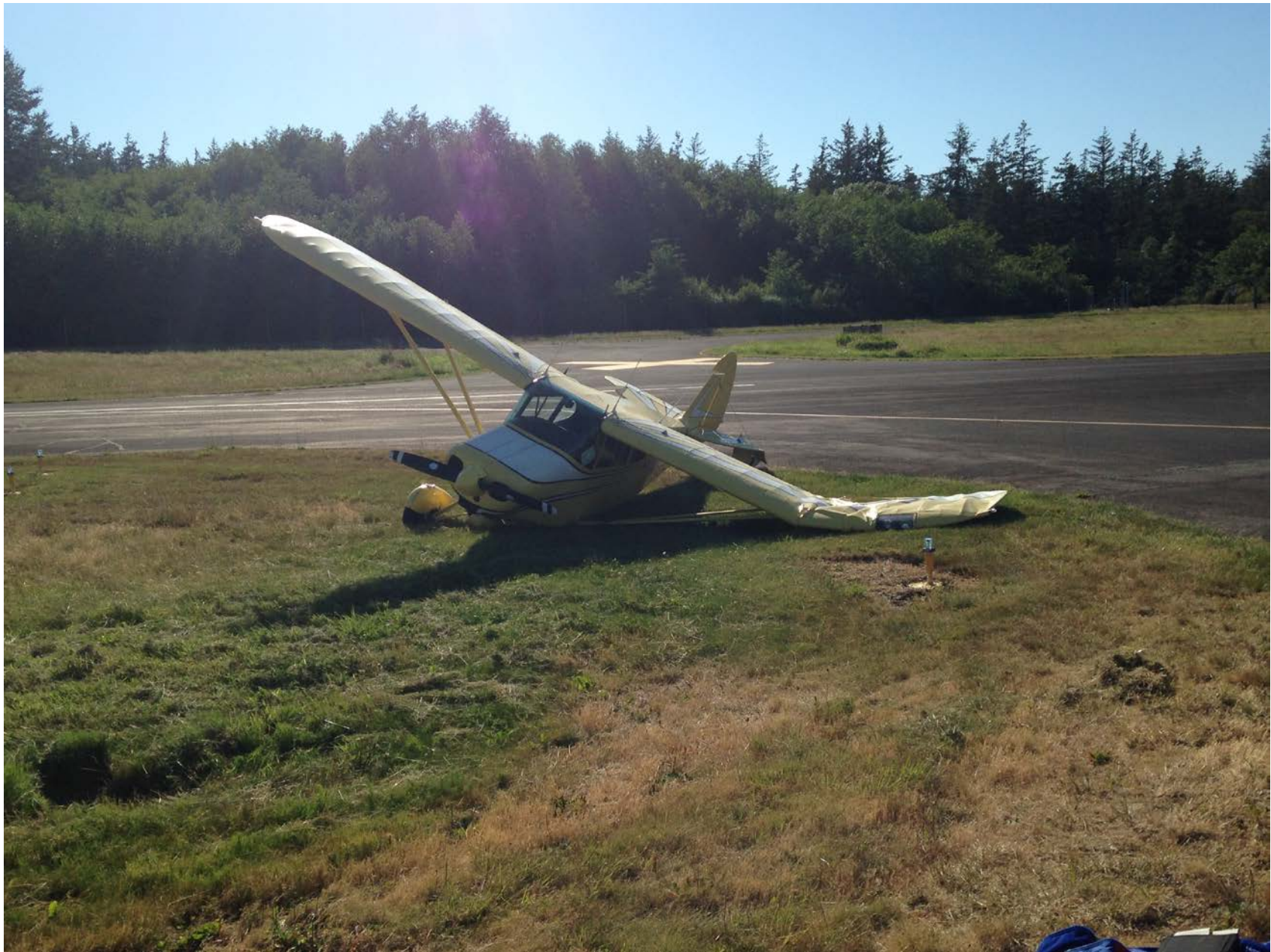
Photo 1 – View of damage to left wing (courtesy of the FAA)
