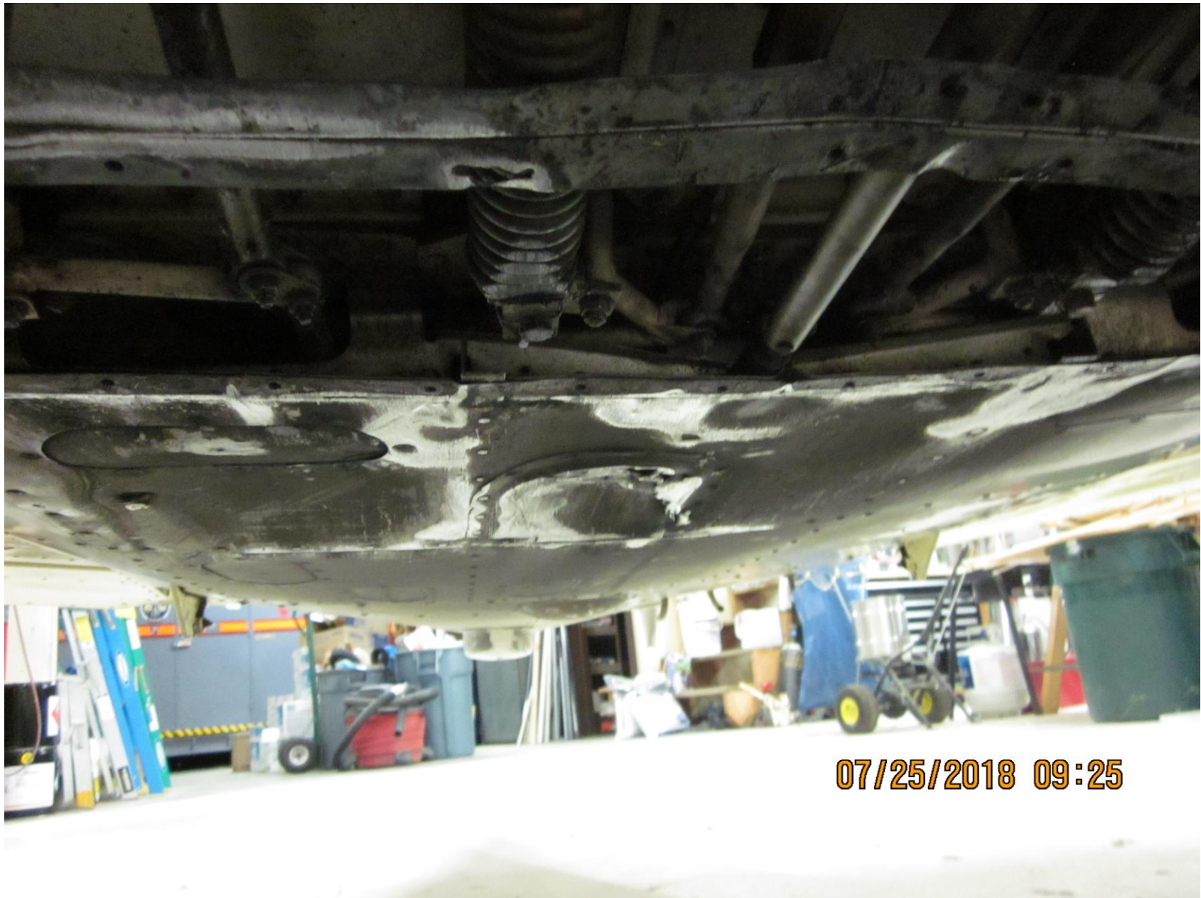
Photo 2 – View of damaged fuselage belly with skin removed (Photo courtesy of the FAA)
