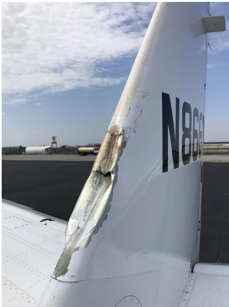
Photo 1 – View of damaged vertical stabilizer (Photo courtesy of the Operator)
