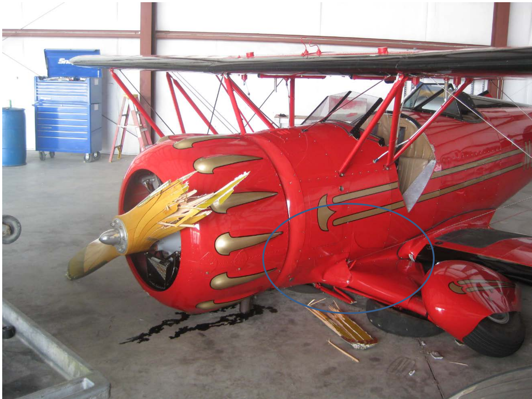
Photo 1 – View of damage to lower fuselage (Photo courtesy of the FAA)
