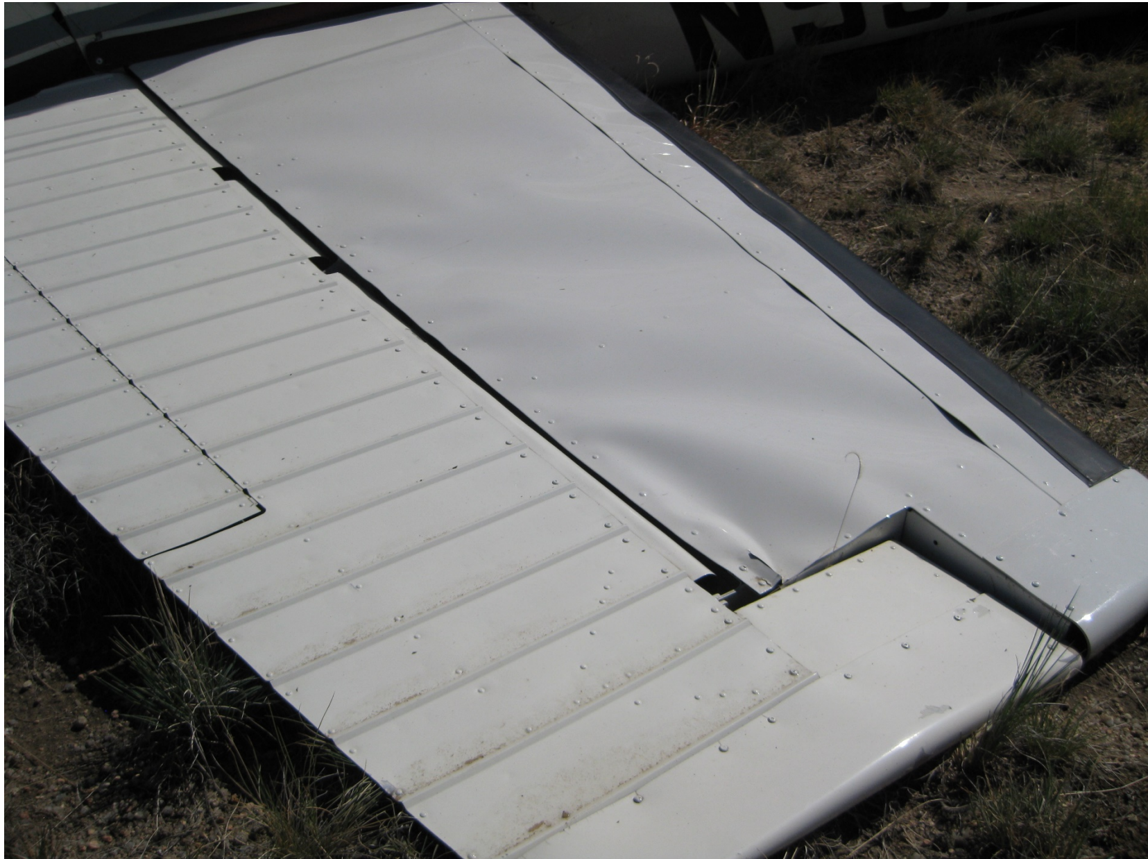
Photo 1 – View of damaged right horizontal stabilizer (Photo courtesy of the FAA)
