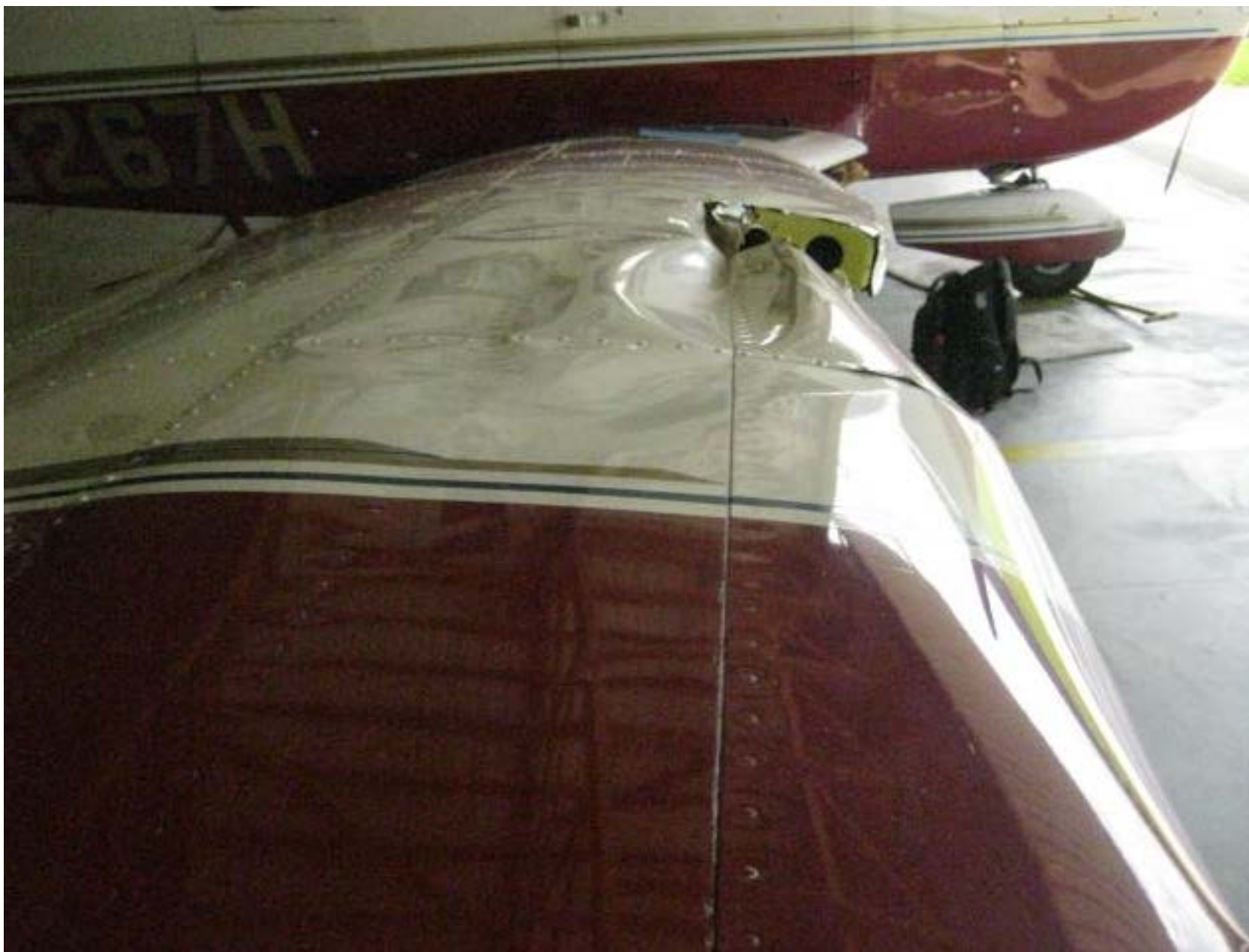
Photo 1 – View of damage to the right wing forward spar (Courtesy of FAA)
