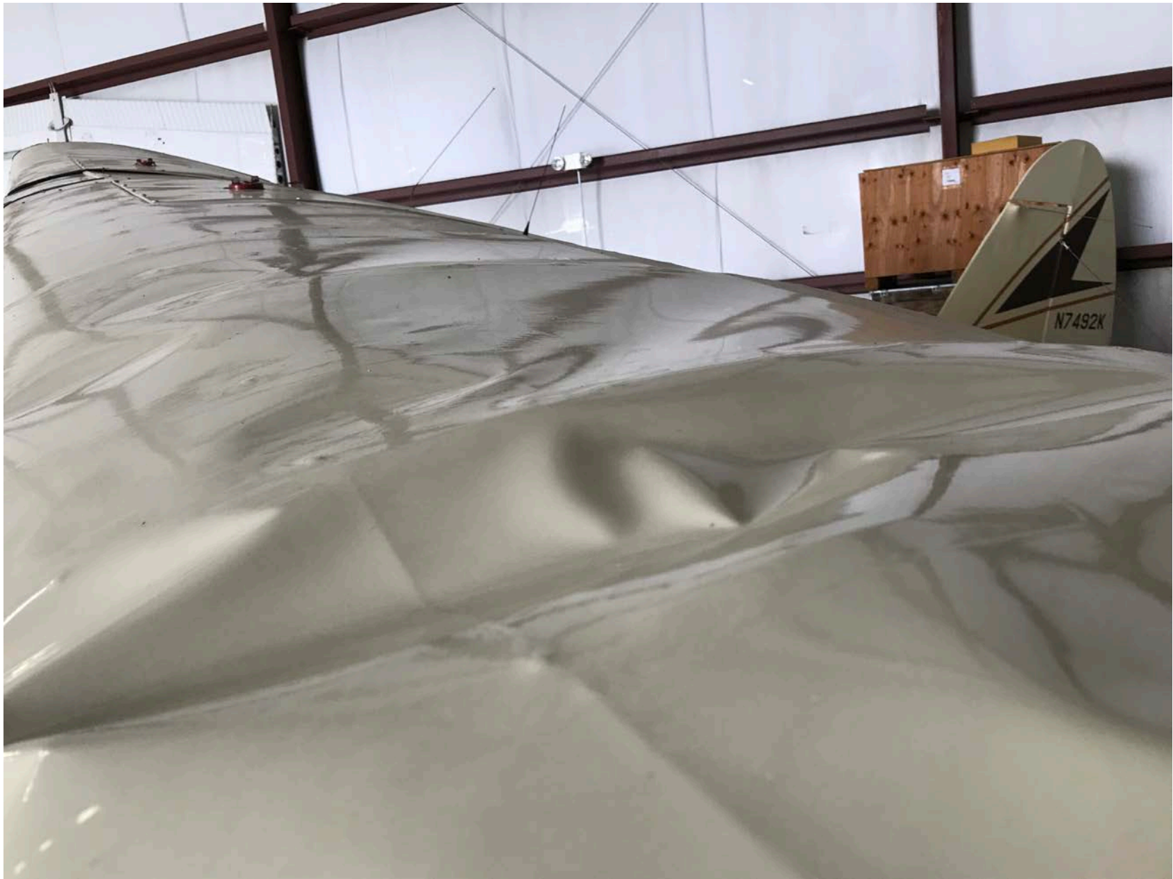
Photo 2 – Close up view of damage to left wing (courtesy of the FAA)
