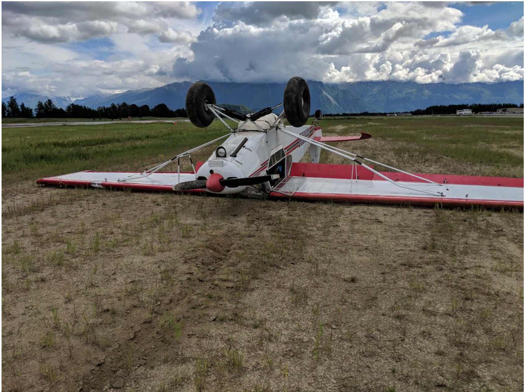
Photo 1 – View of damage to left and right wing lift struts (Photo courtesy of the FAA)
