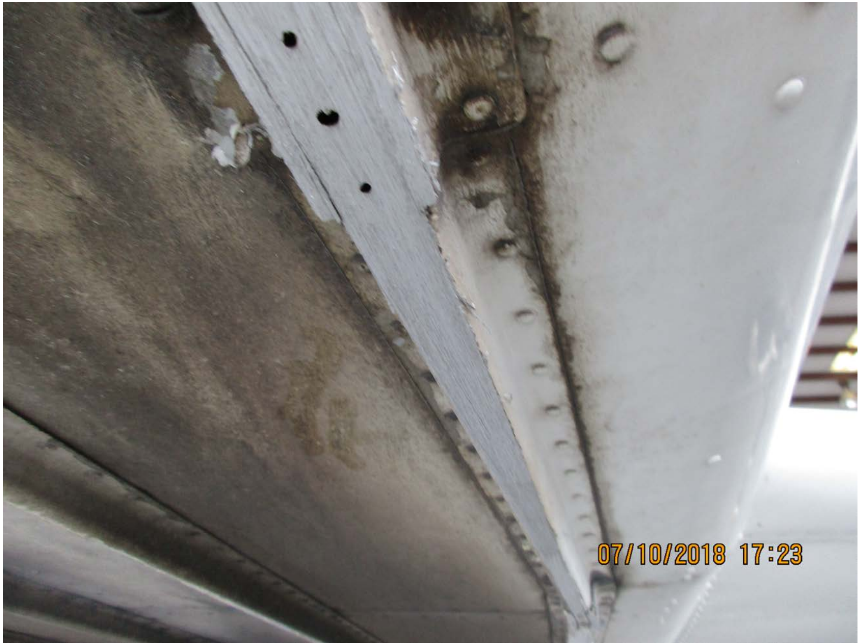
Photo 2 – View of damaged exterior longerons on the lower fuselage (photo courtesy of the FAA)
