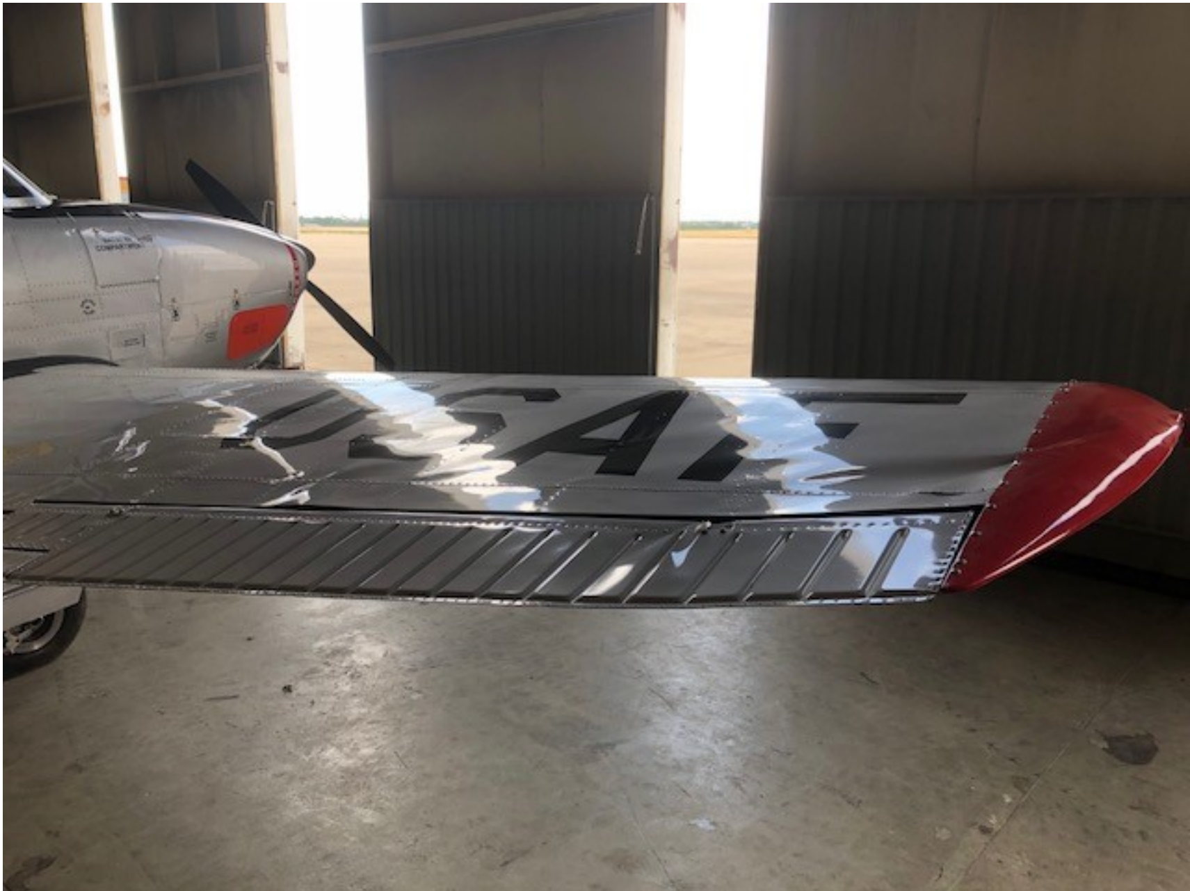
Photo 1 – View of damaged right wing and aileron (Photo courtesy of the FAA)
