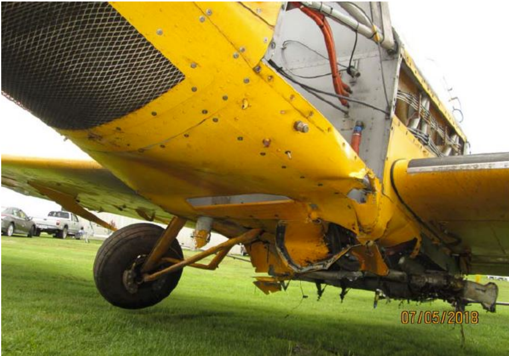
Photo 1 – View of damage to lower fuselage (Courtesy of the FAA)
