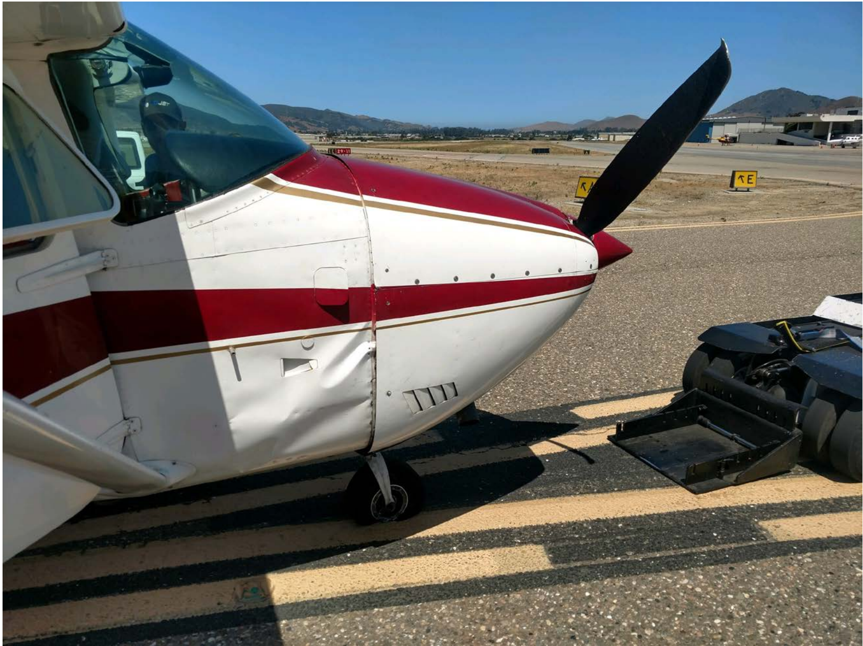
Photo 2 – View of damage to the lower right fuselage stringers (Courtesy of Operator)
