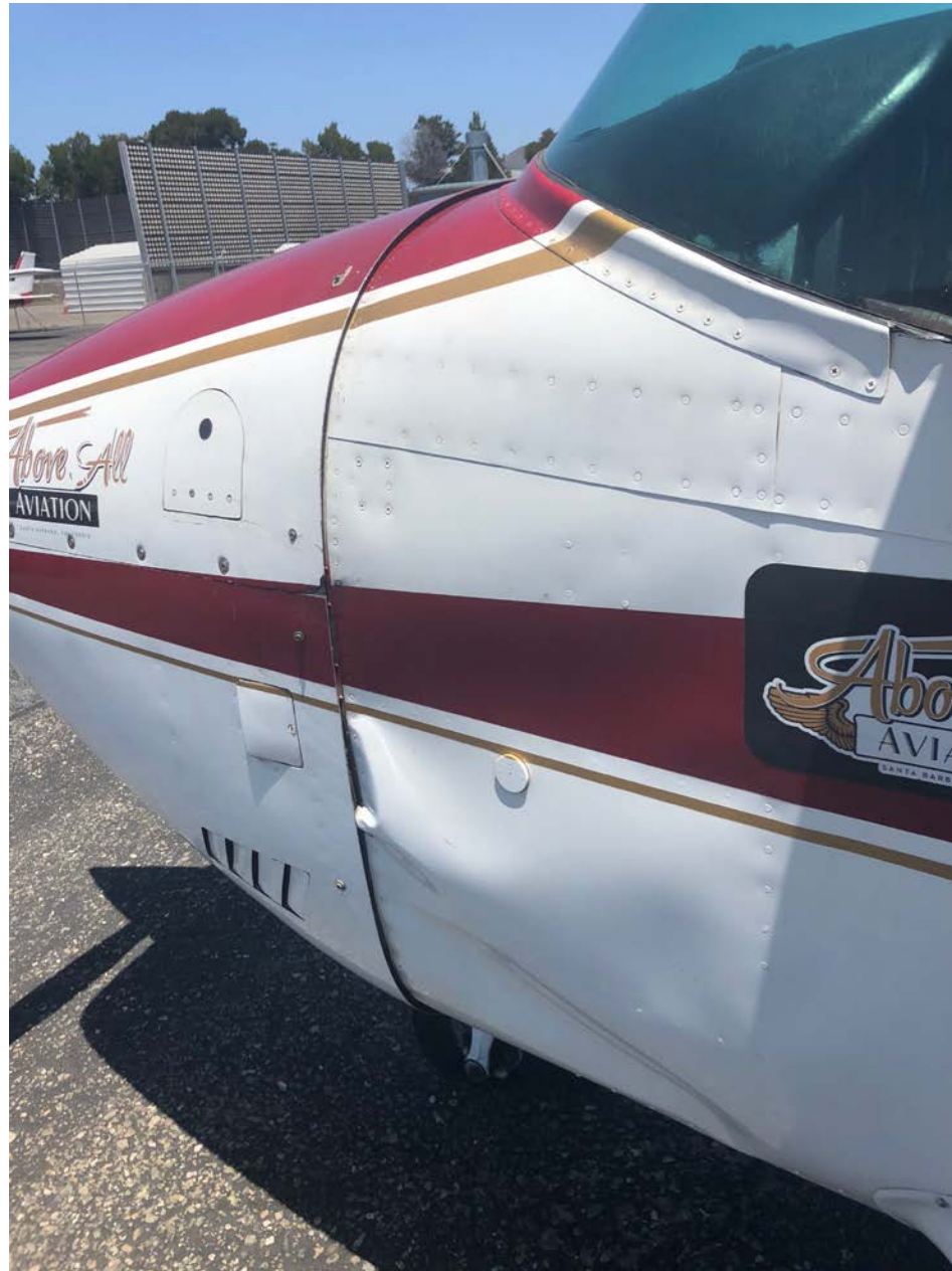
Photo 1 – View of damage to the lower left fuselage stringer (Courtesy of Operator)
