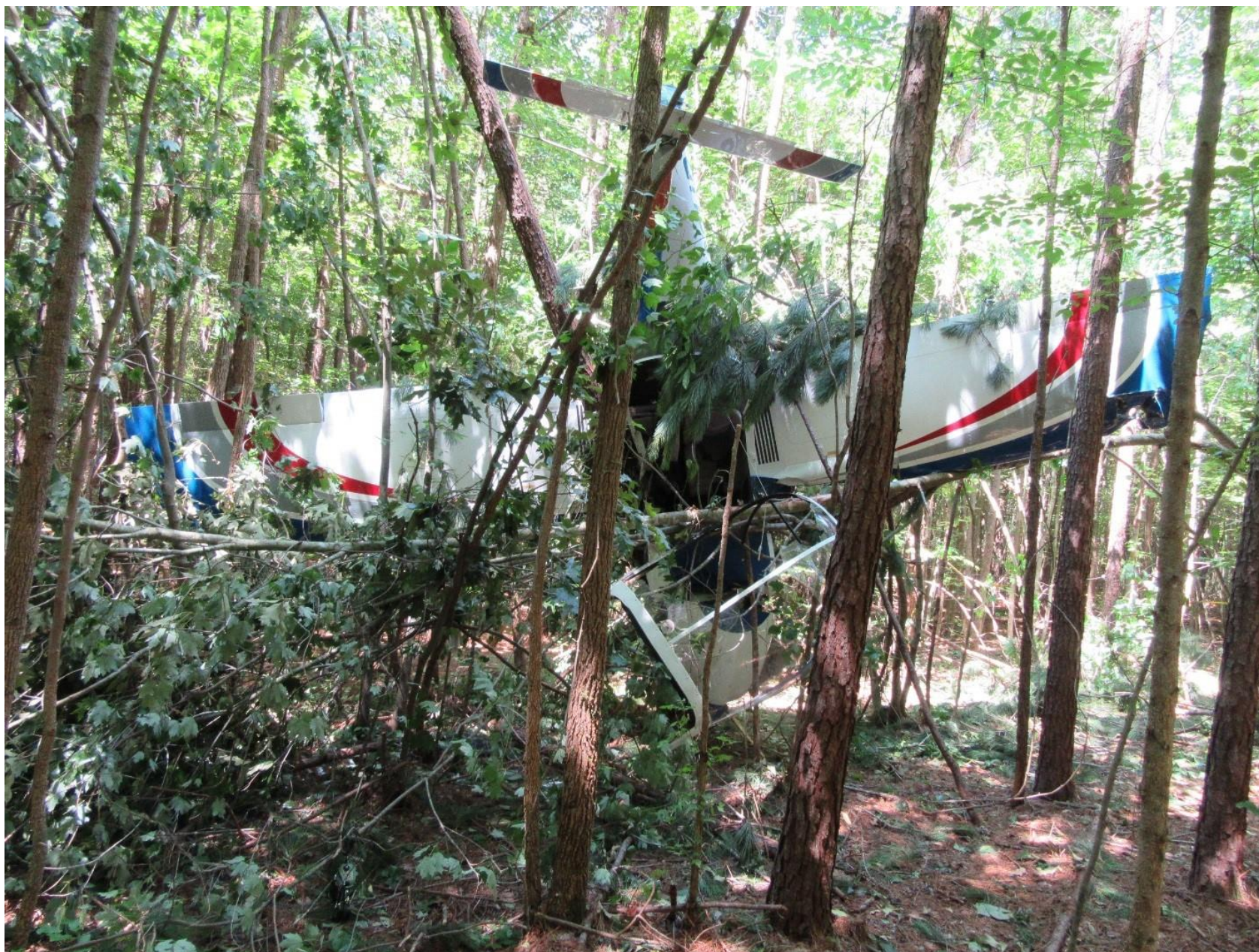
Photo 1 – View of left wing damage (Courtesy of the FAA)
