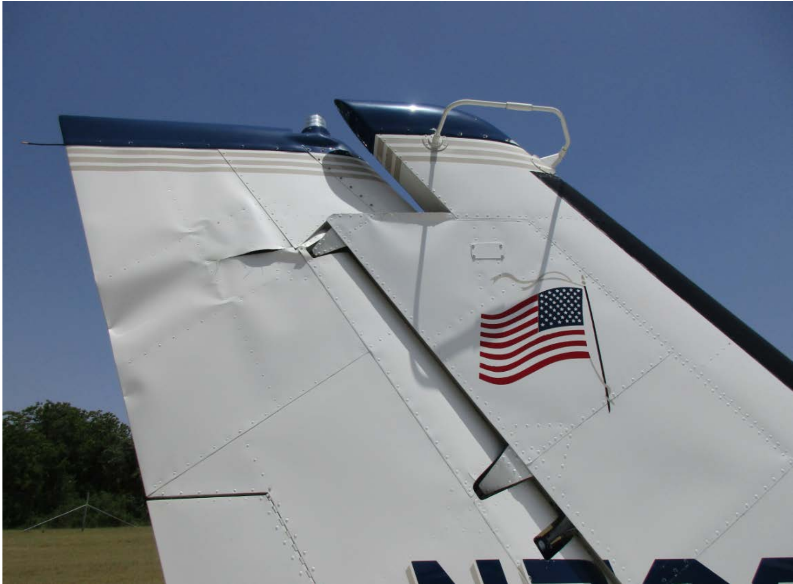
Photo 3 – View of damaged rudder (Photo Courtesy of FAA)
