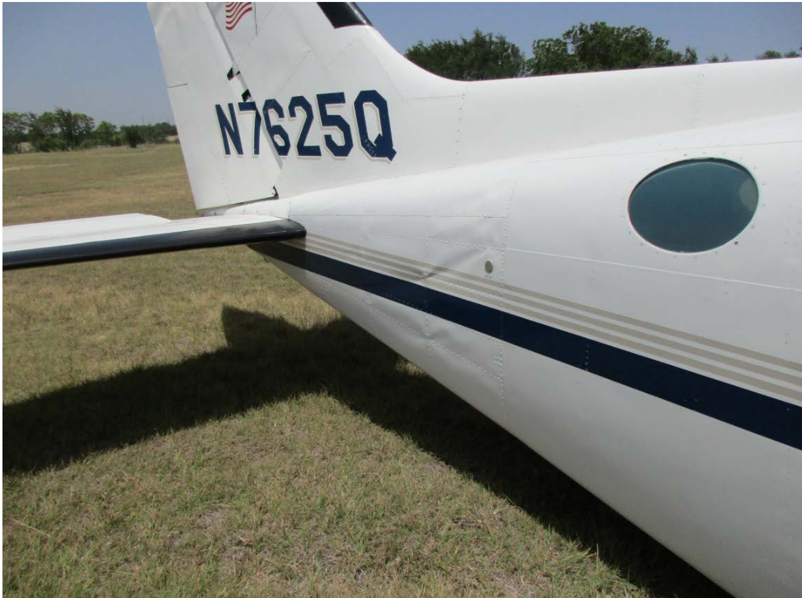
Photo 2 – View of damaged tail cone (Photo courtesy of FAA)
