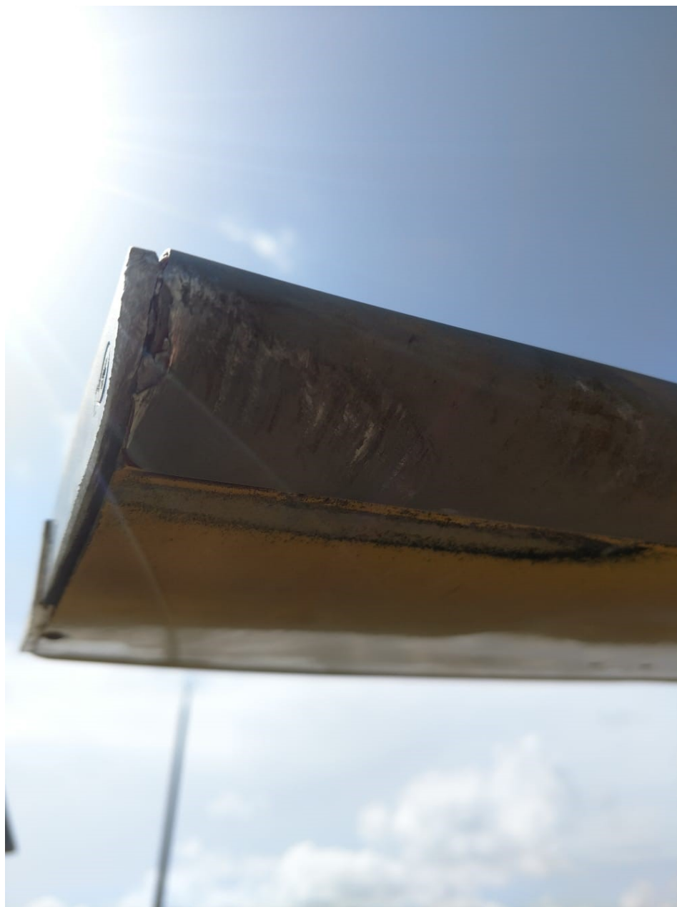
Photo 1 – View of damage to the outboard section of the main rotor blade (Courtesy of FAA)
