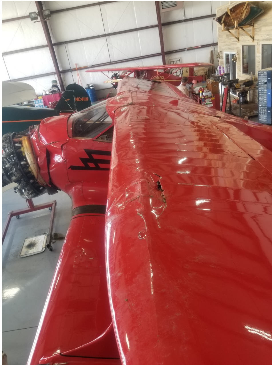
Photo 2 – View of damaged fuselage and left upper wing (Photo courtesy of the FAA)
