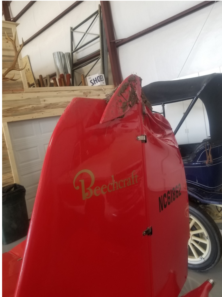
Photo 3 – View of damaged rudder (Photo courtesy of the FAA)
