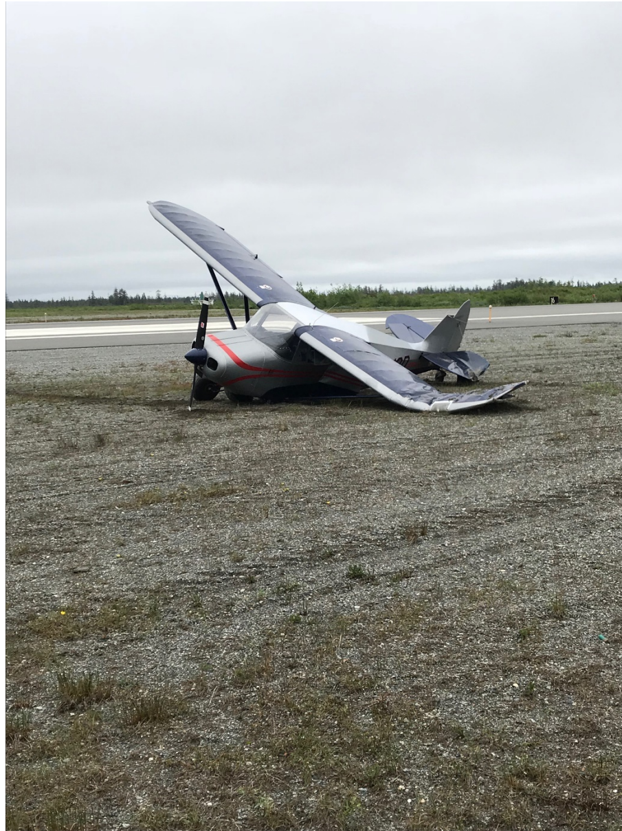
Photo 2 – View of damaged left wing (Photo courtesy of the Alaska DOT)
