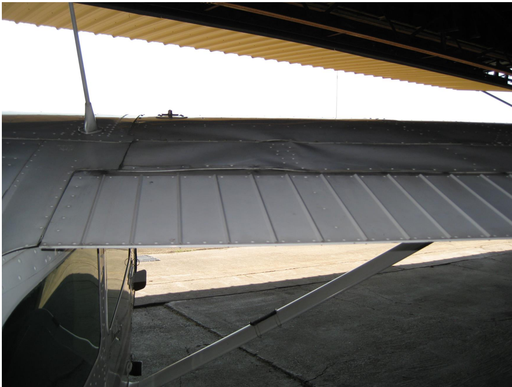
Photo 1 – Rear view of damaged right wing (Photo courtesy of the FAA)
