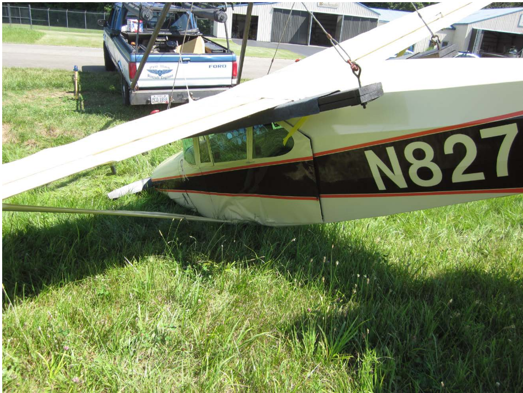
Photo 1 – View of left lower fuselage damage (courtesy of the FAA)
