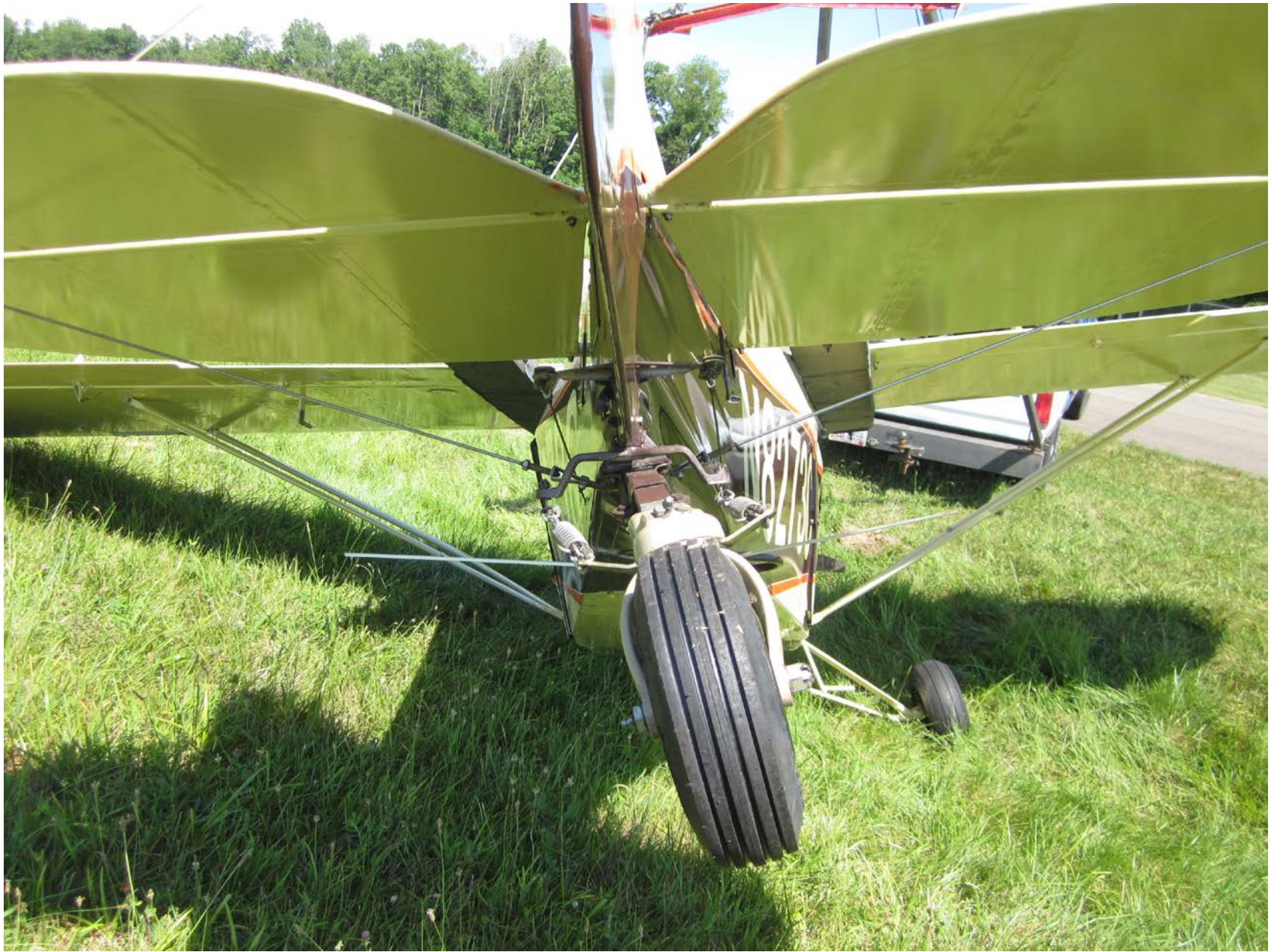
Photo 2 – View of bent tailwheel (courtesy of the FAA)
