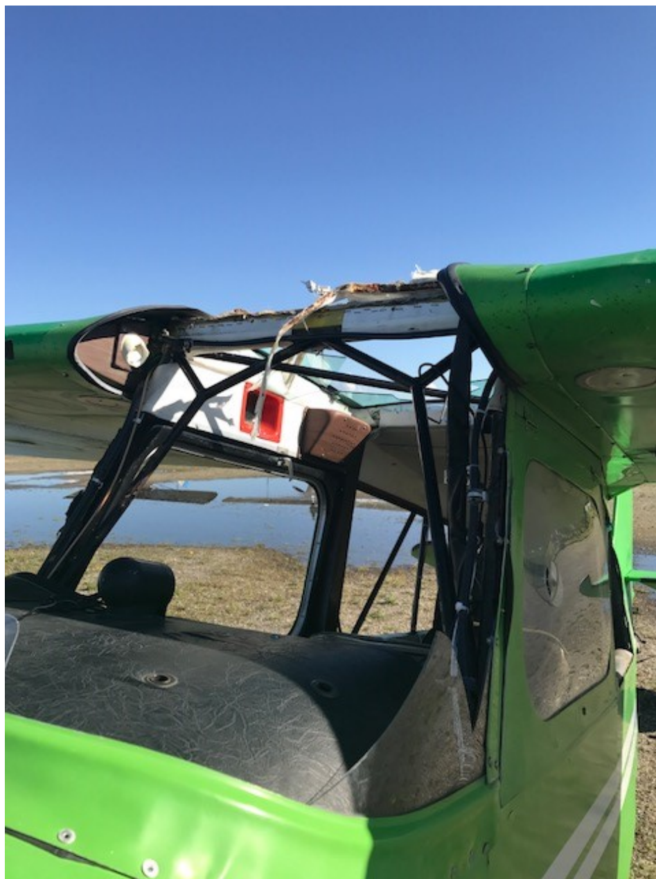
Photo 1 – View of missing windscreen, windows, and greenhouse (Courtesy of FAA)
