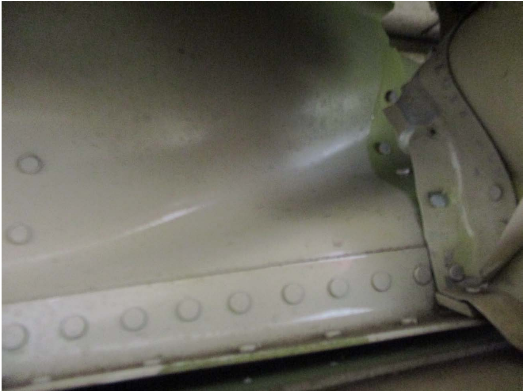
Photo 2 – View of damage to the right wing rear spar (Courtesy of FAA)
