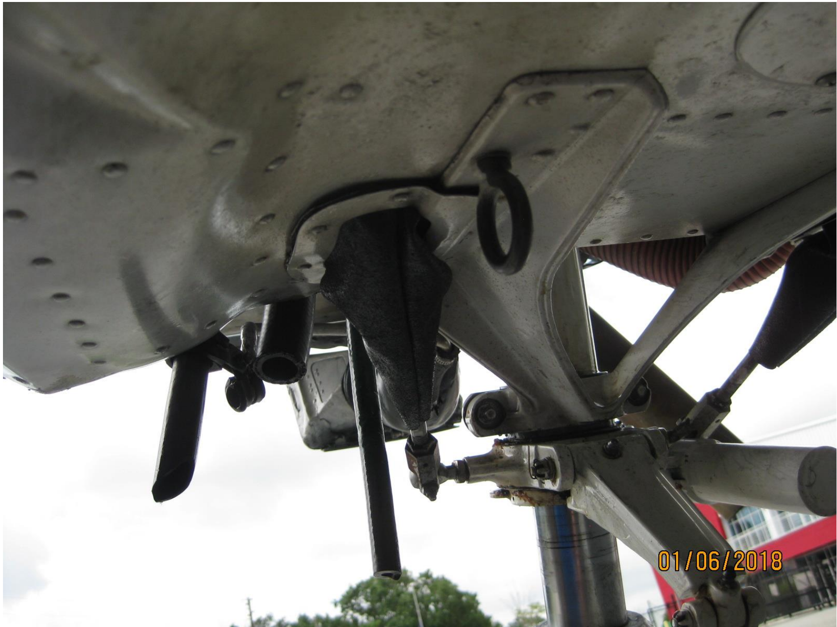
Photo 1 – View of damaged bottom forward fuselage (Photo courtesy of the FAA)
