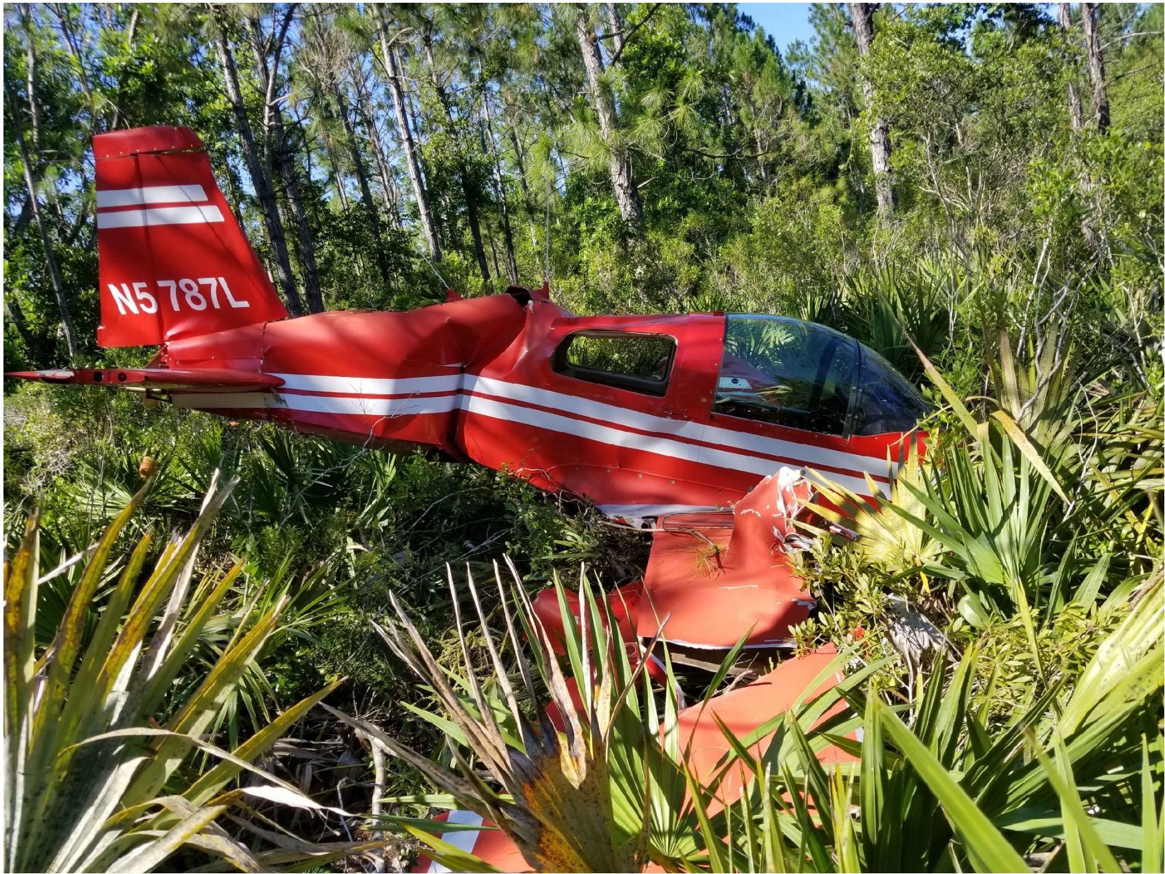
Photo 1 – view of damage to right wing and fuselage (photo courtesy of the pilot)
