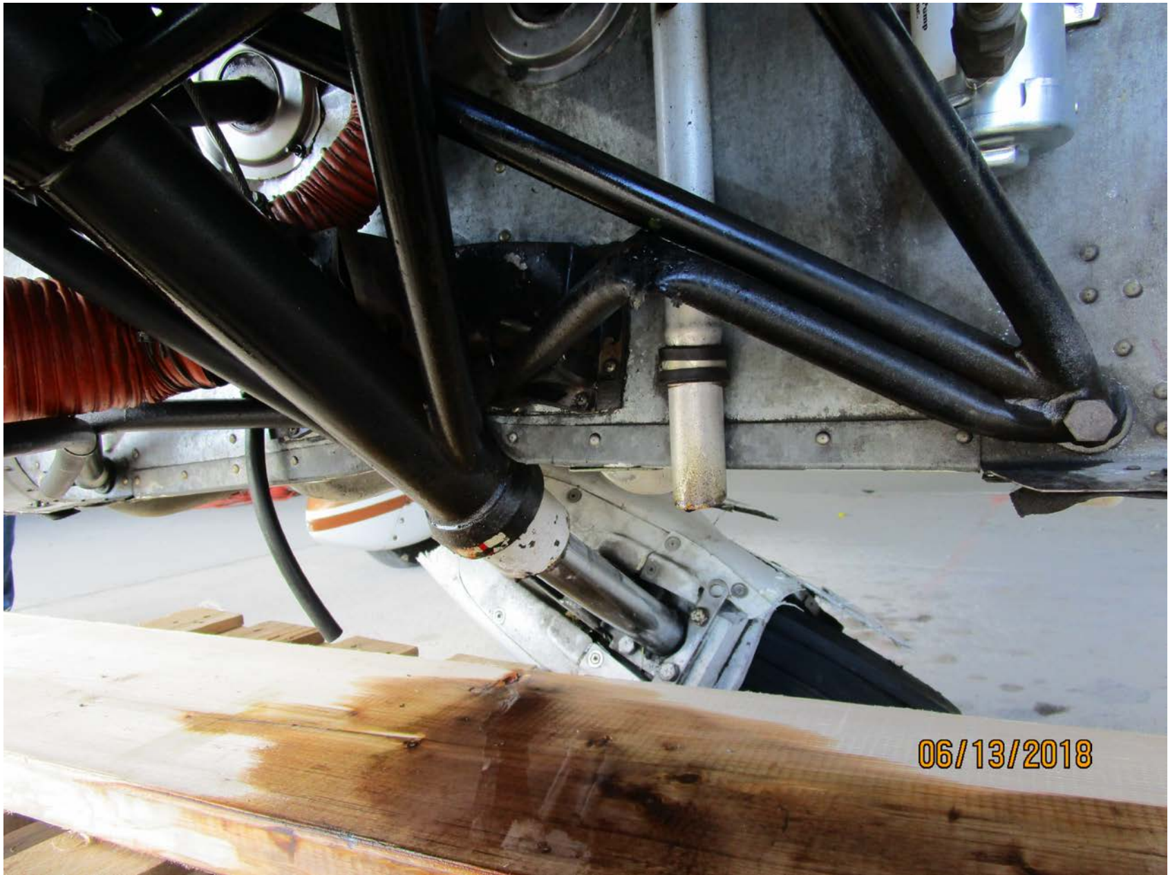
Photo 1 – View of damage to the engine mount (Courtesy of FAA)
