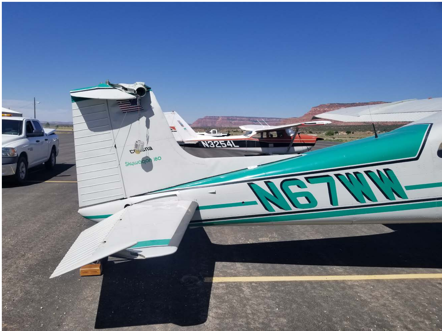
Photo 1 – View of damage to the vertical stabilizer and rudder (Courtesy of FAA)
