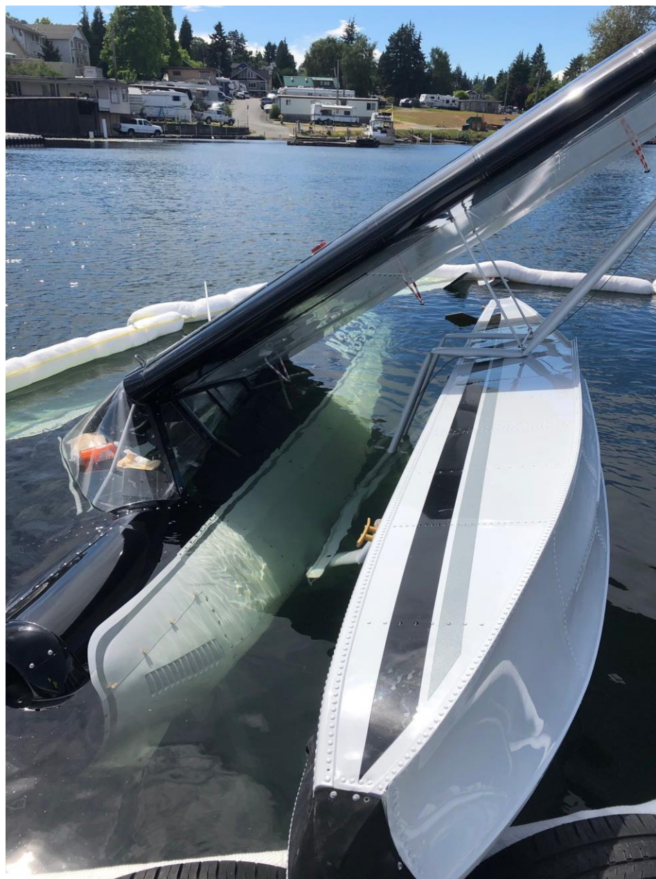
Photo 1 – View of damaged left wing lift strut (Photo courtesy of the FAA)
