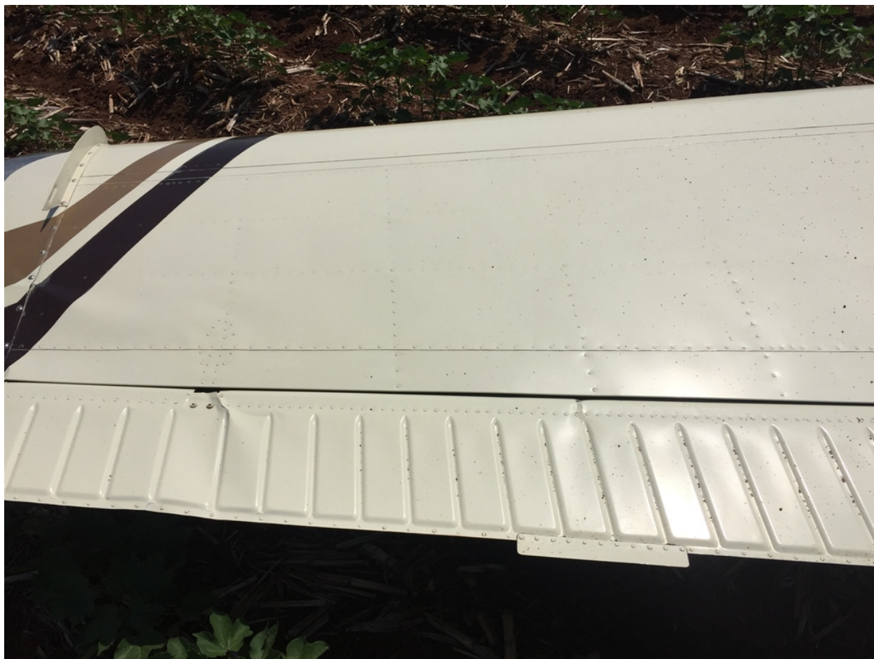
Photo 2. Damage to left aileron (photo courtesy of the FAA).
