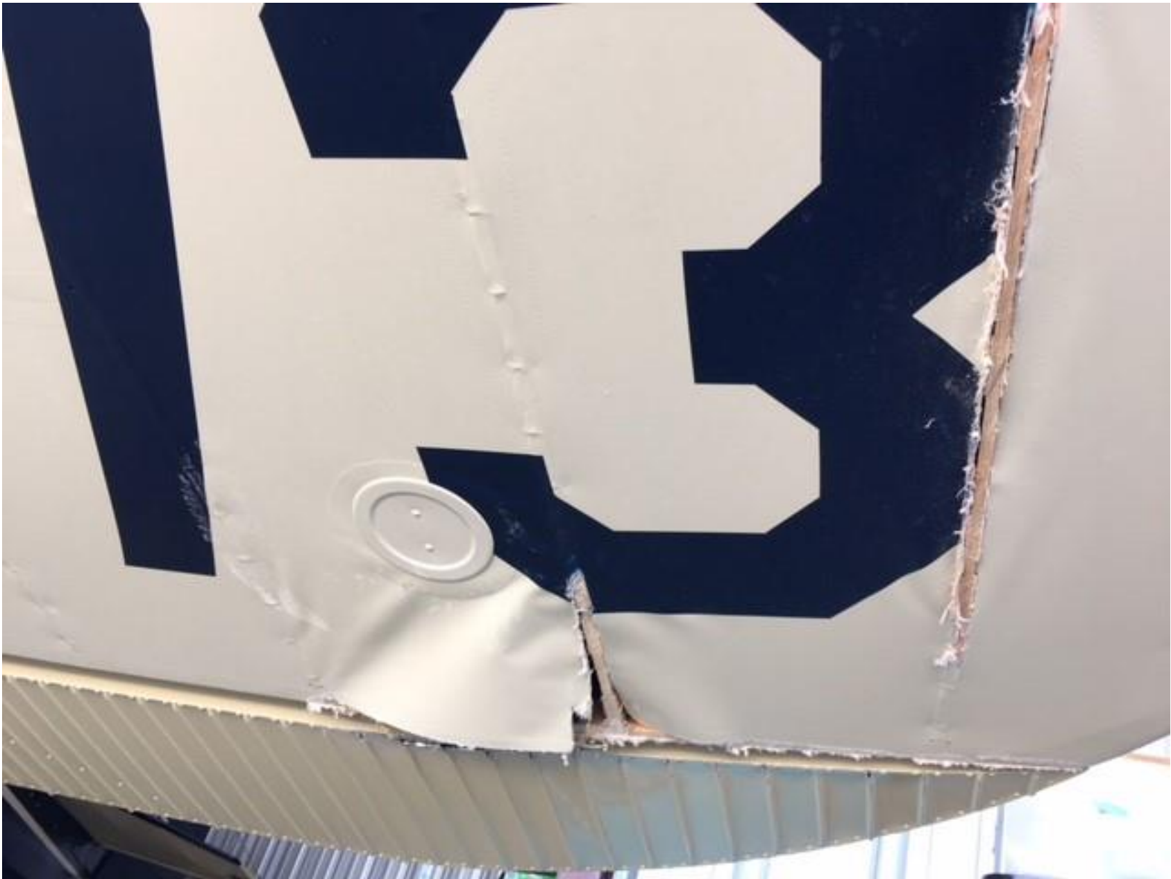
Photo 1 – Bottom view of damaged lower left wing (Photo courtesy of the FAA)
