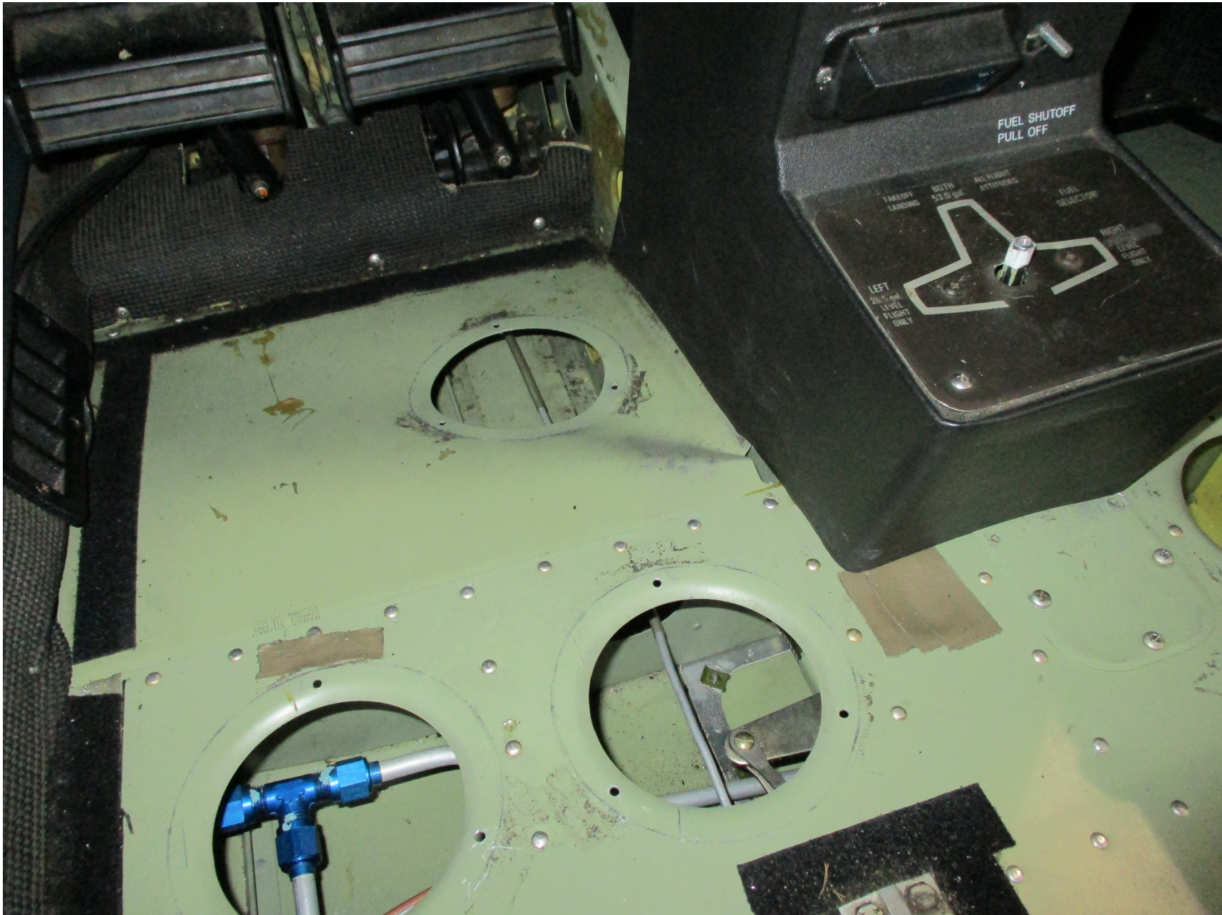
Photo 1 – View of damaged floorboards (Photo courtesy of the FAA)
