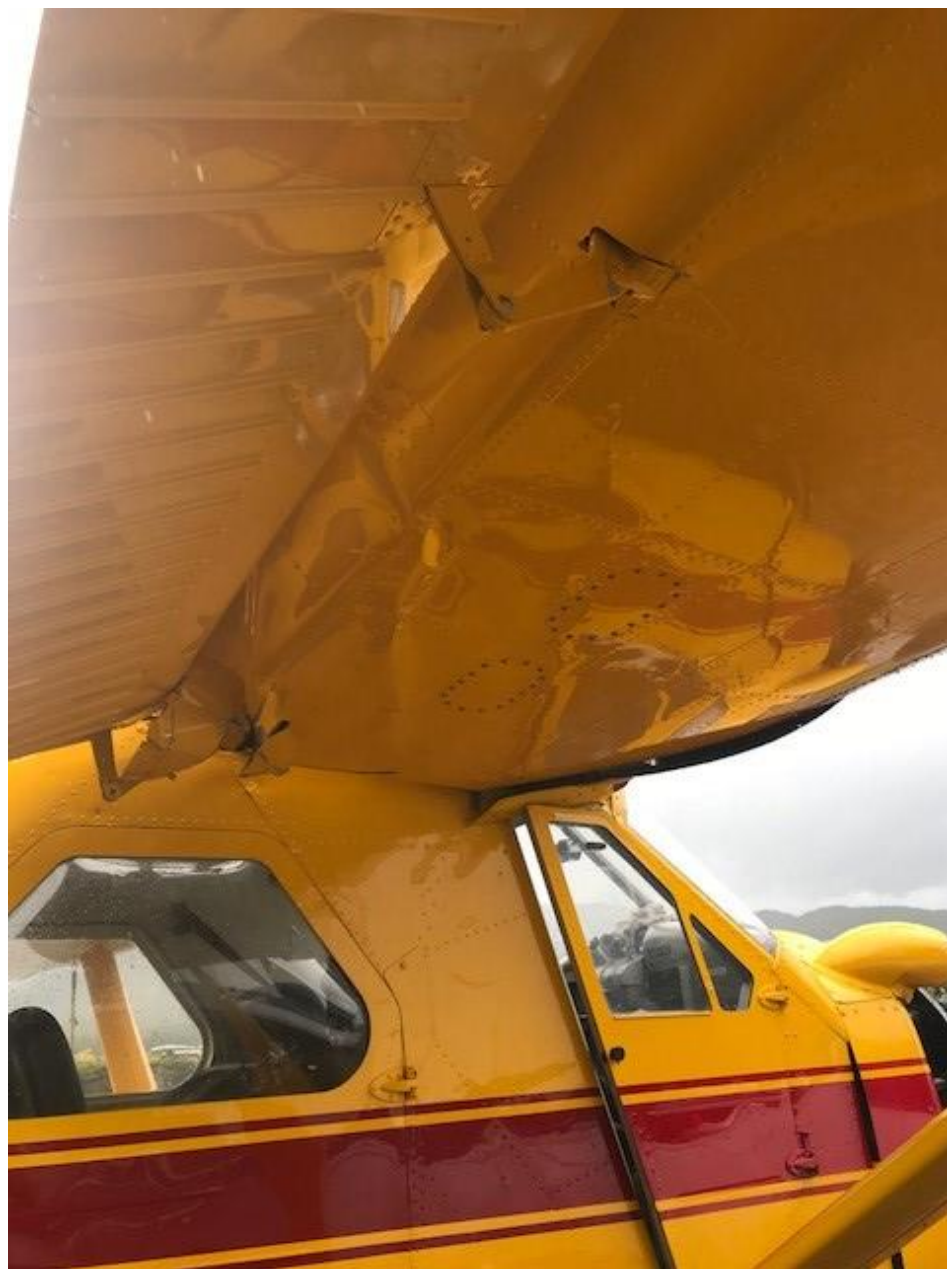
Photo 3 – View of damaged right wing root (Photo courtesy of the FAA)
