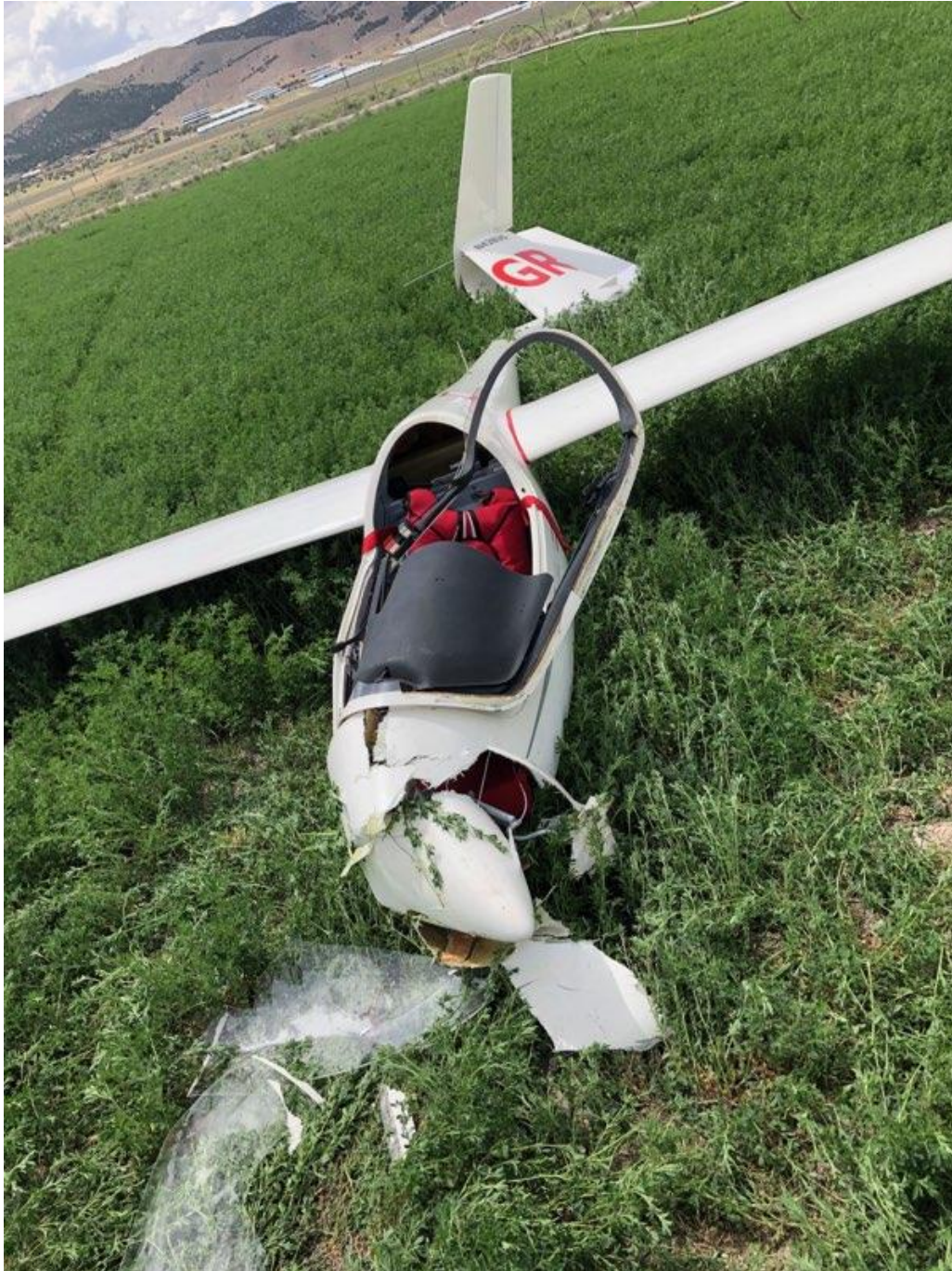
Photo 1- View of damage to fuselage and empennage (photo courtesy of FAA)
