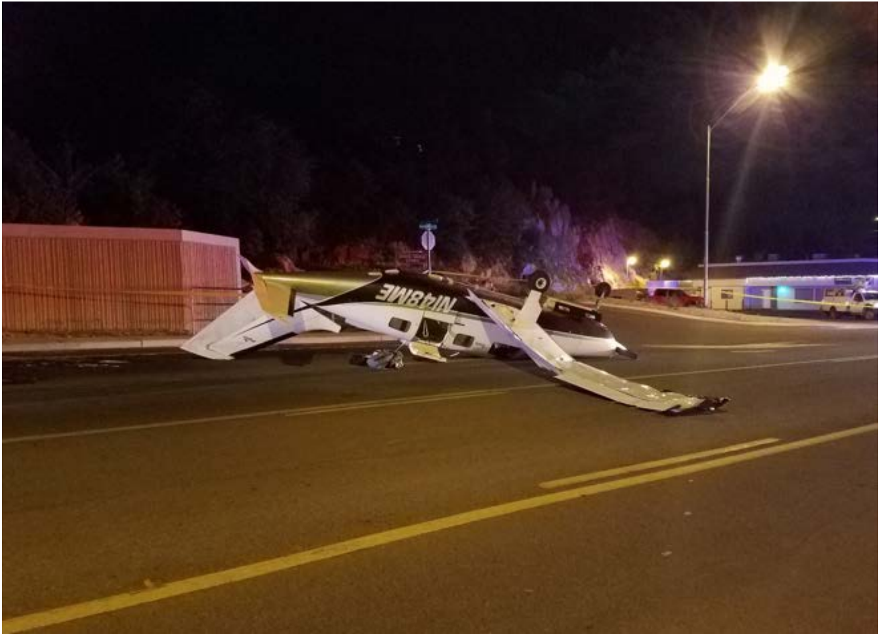
Photo 1 – View of damage to the left wing, the vertical stabilizer, and rudder (Courtesy of FAA)
