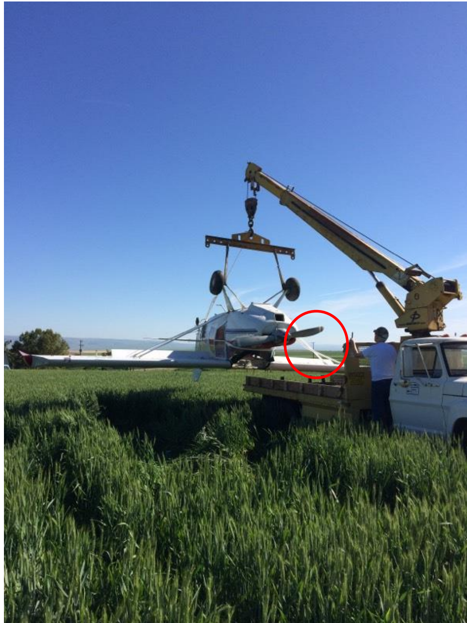
Photo 1 – View of damage to right lift strut (photo courtesy of the pilot)
