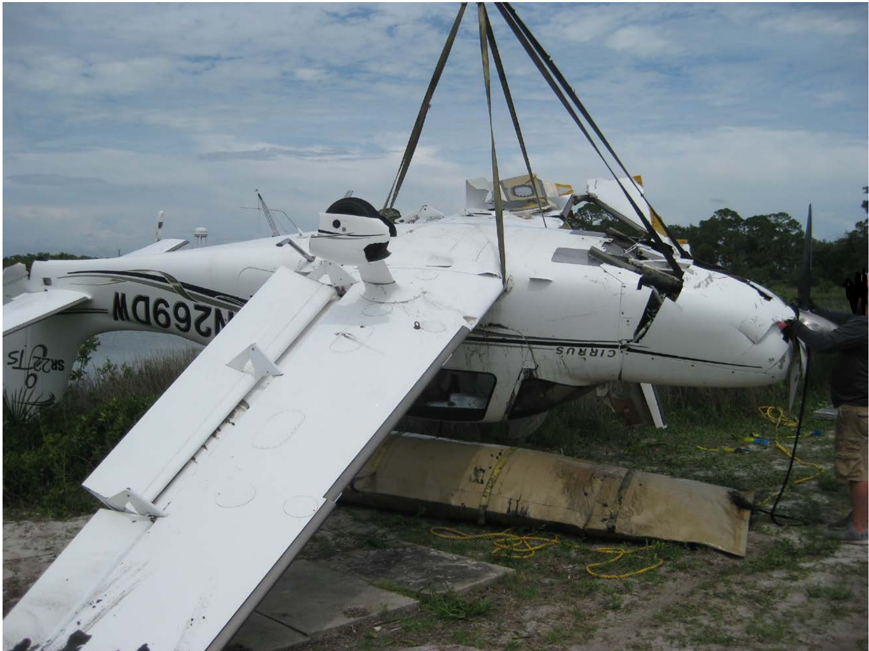
Photo 2 – View of the left wing and damage to the right wing (Courtesy of FAA)
