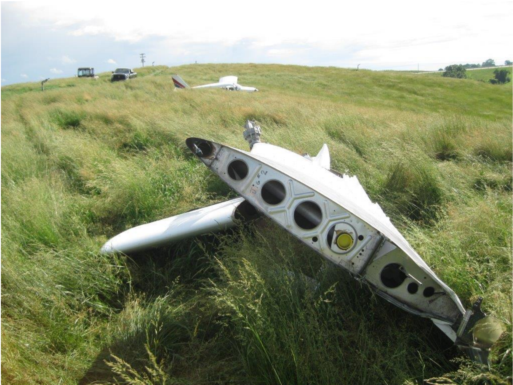
Photo 1 – View of accident airplane with right wing separated (Photo courtesy of the FAA)
