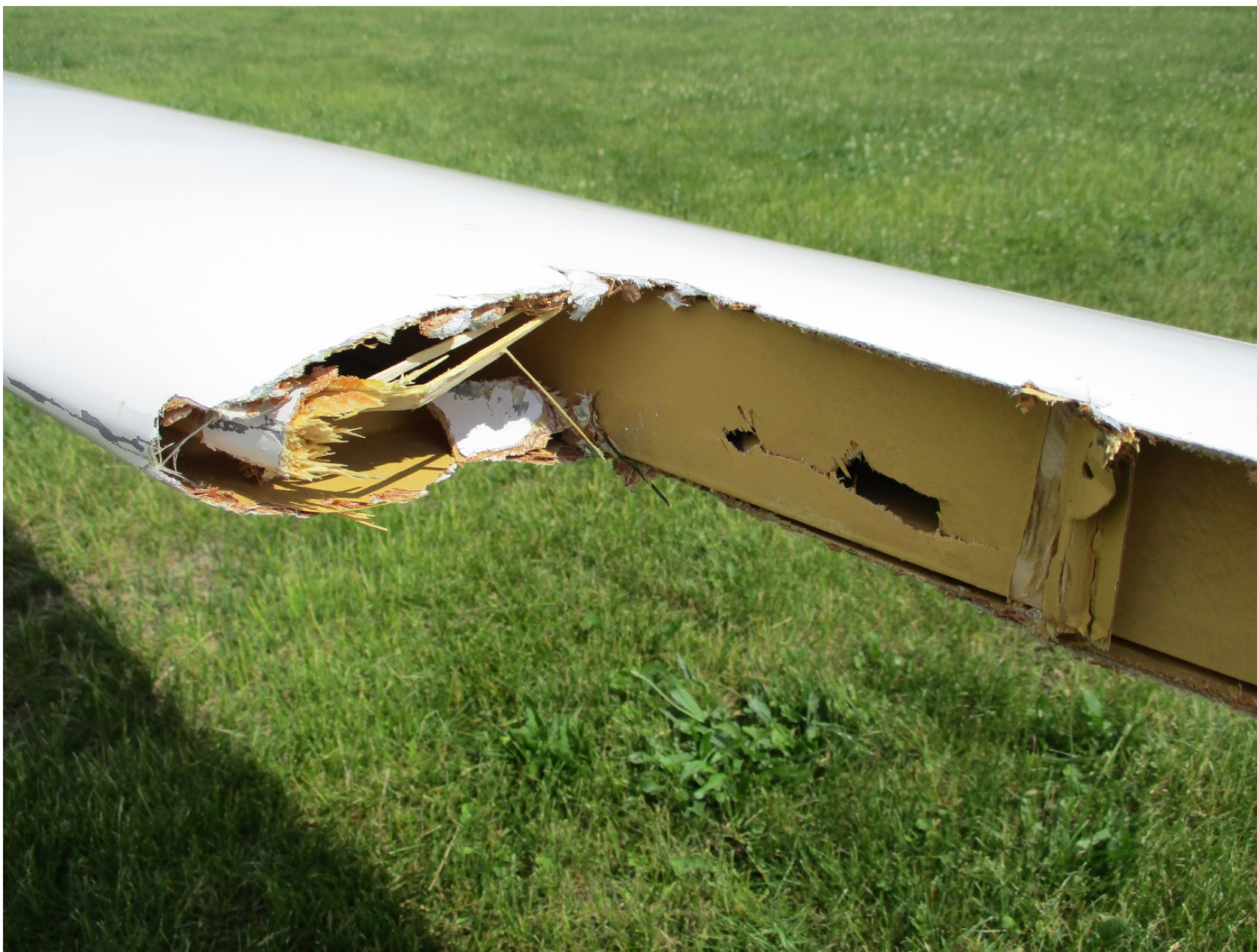
Photo 3 – View of damage to outboard left wing (Courtesy of FAA)
