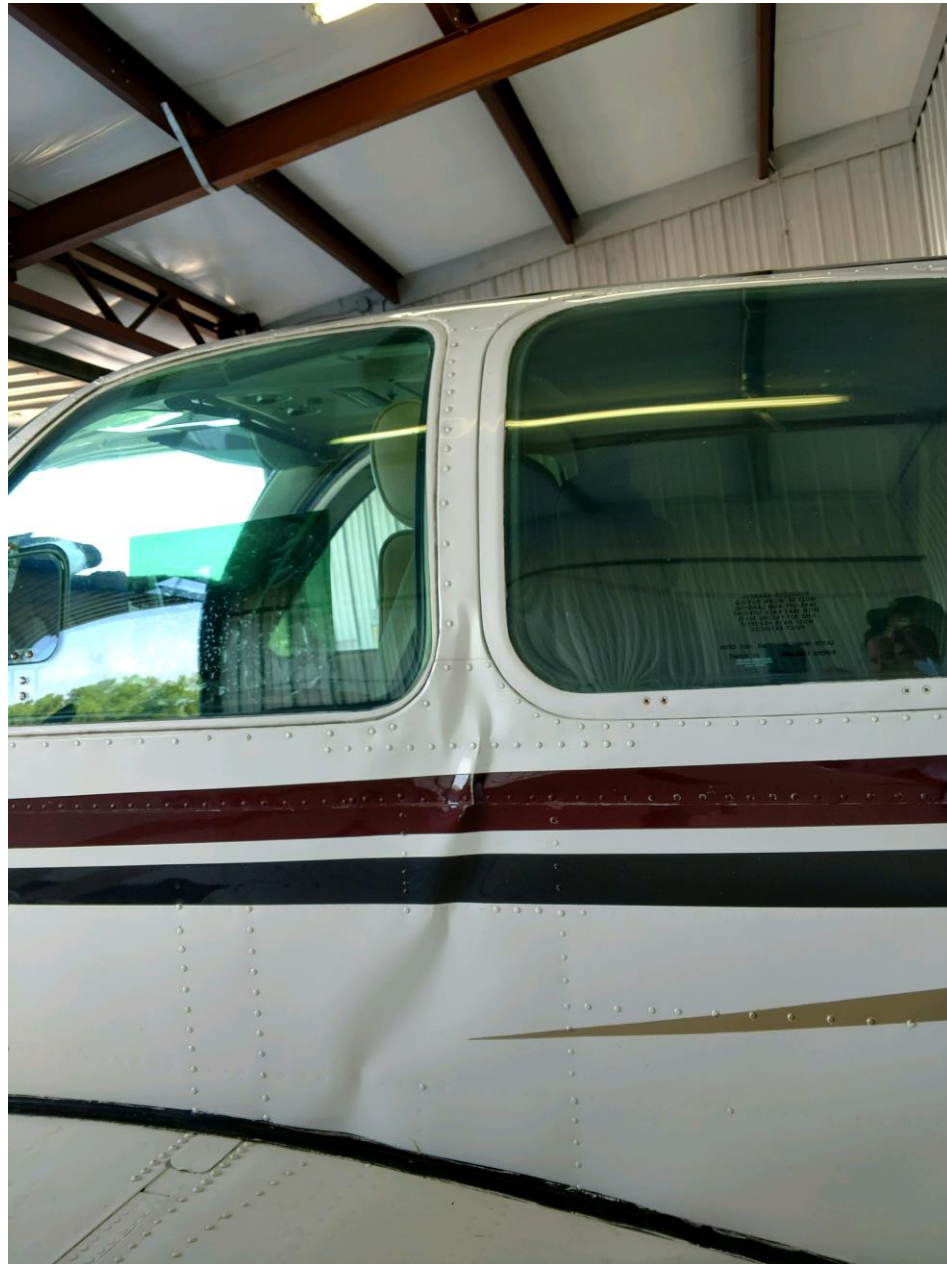
Photo 1 – View of left side fuselage damage (Photo courtesy of the FAA)
