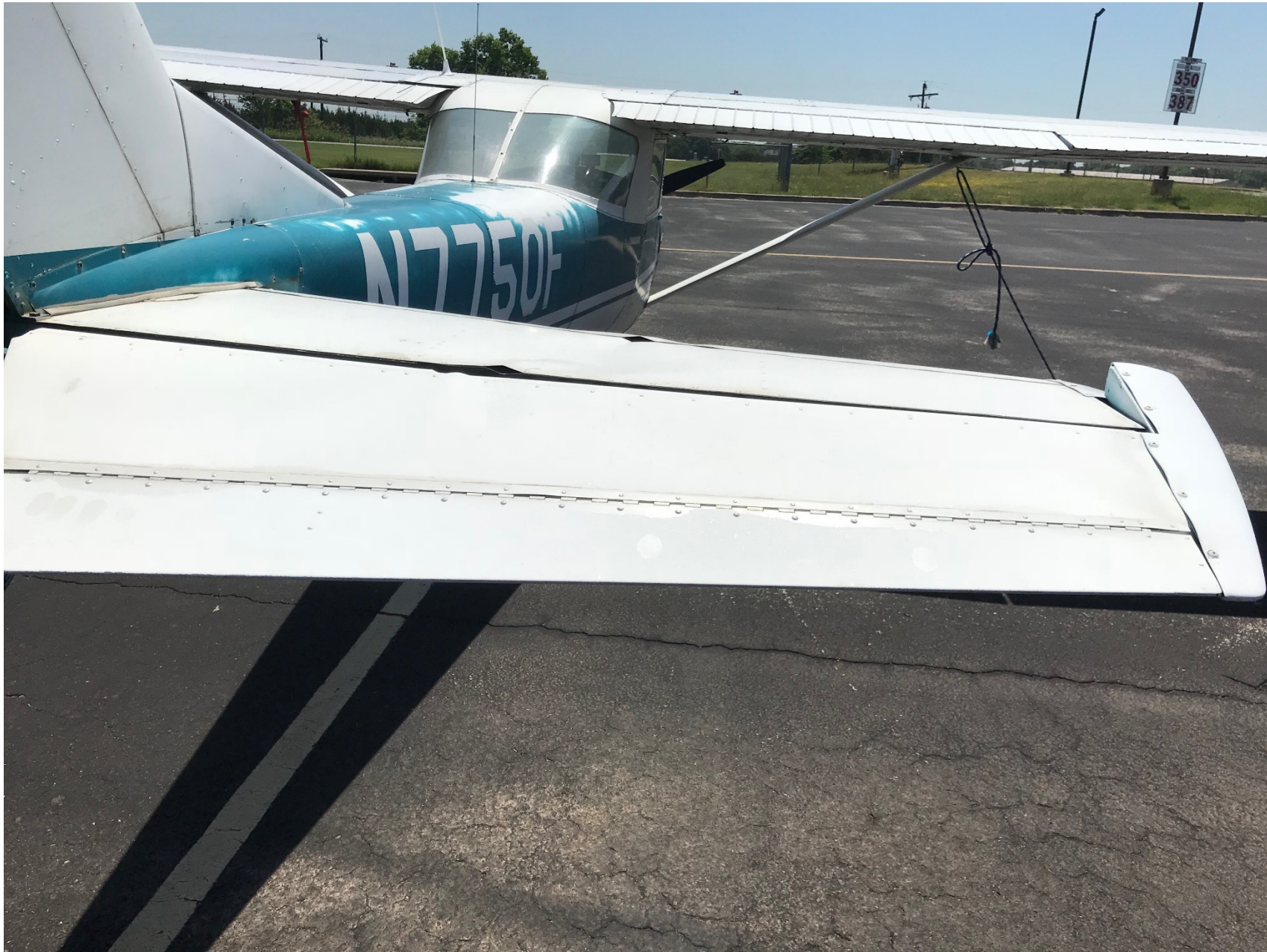
Photo 2 – View of damaged right horizontal stabilizer (Photo courtesy of the pilot)
