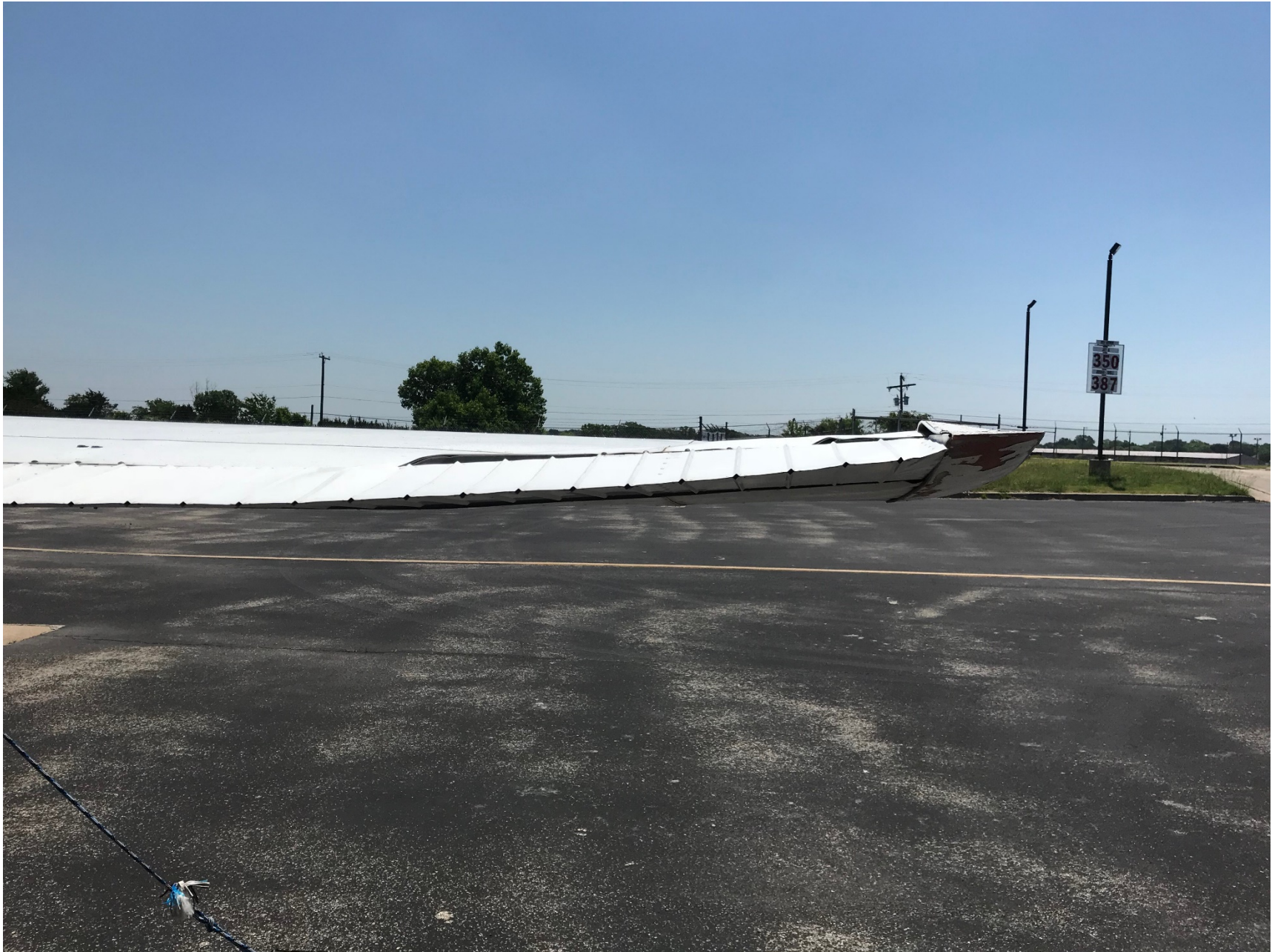
Photo 1 – View of damaged right wing and aileron (Photo courtesy of the pilot)
