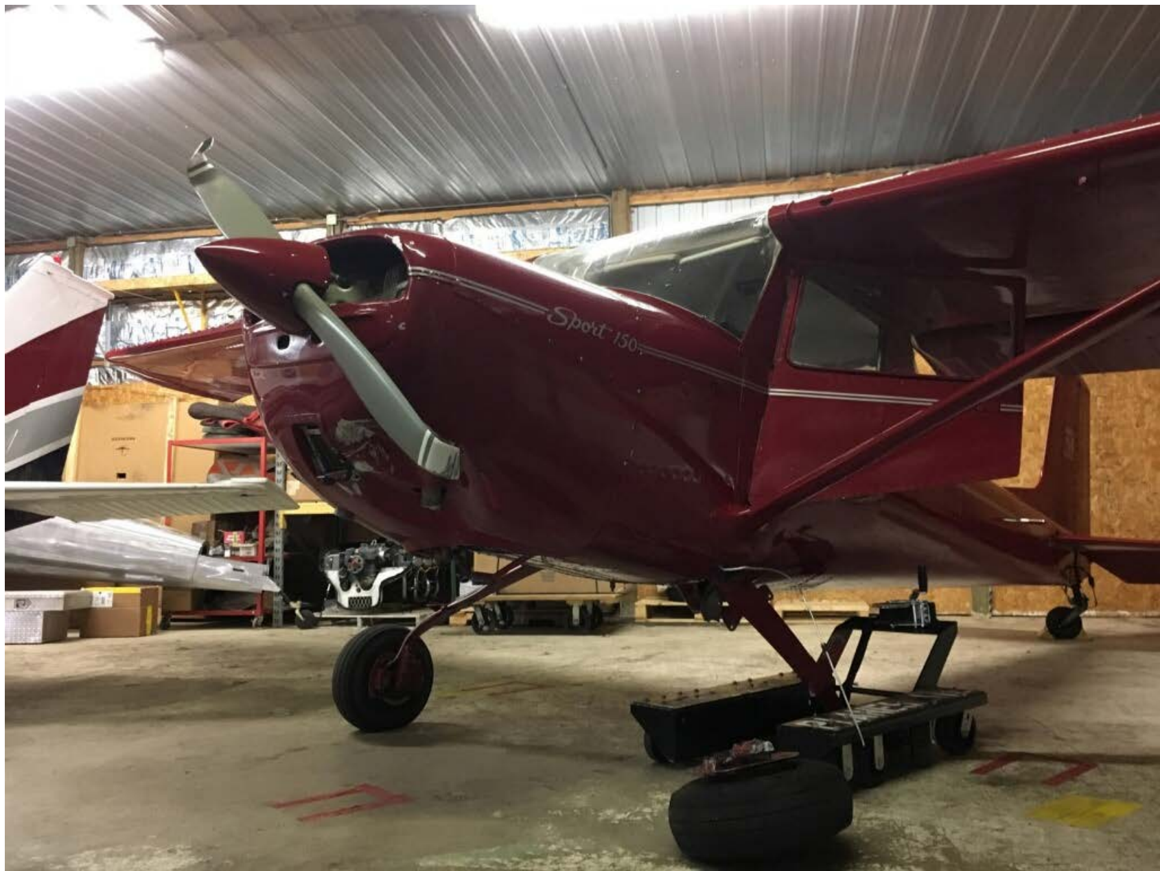
Photo 2 – View of damage to the left main landing gear strut and wheel (Courtesy of FAA)
