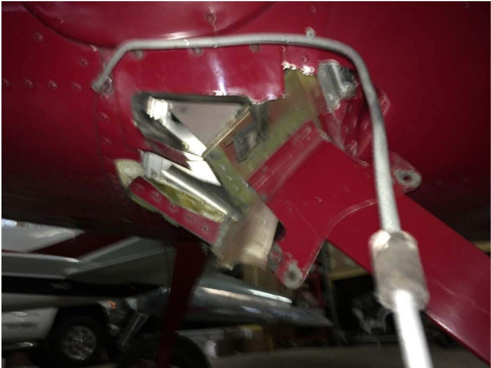
Photo – View of damage to left main landing gear attachment point (Courtesy of FAA)
