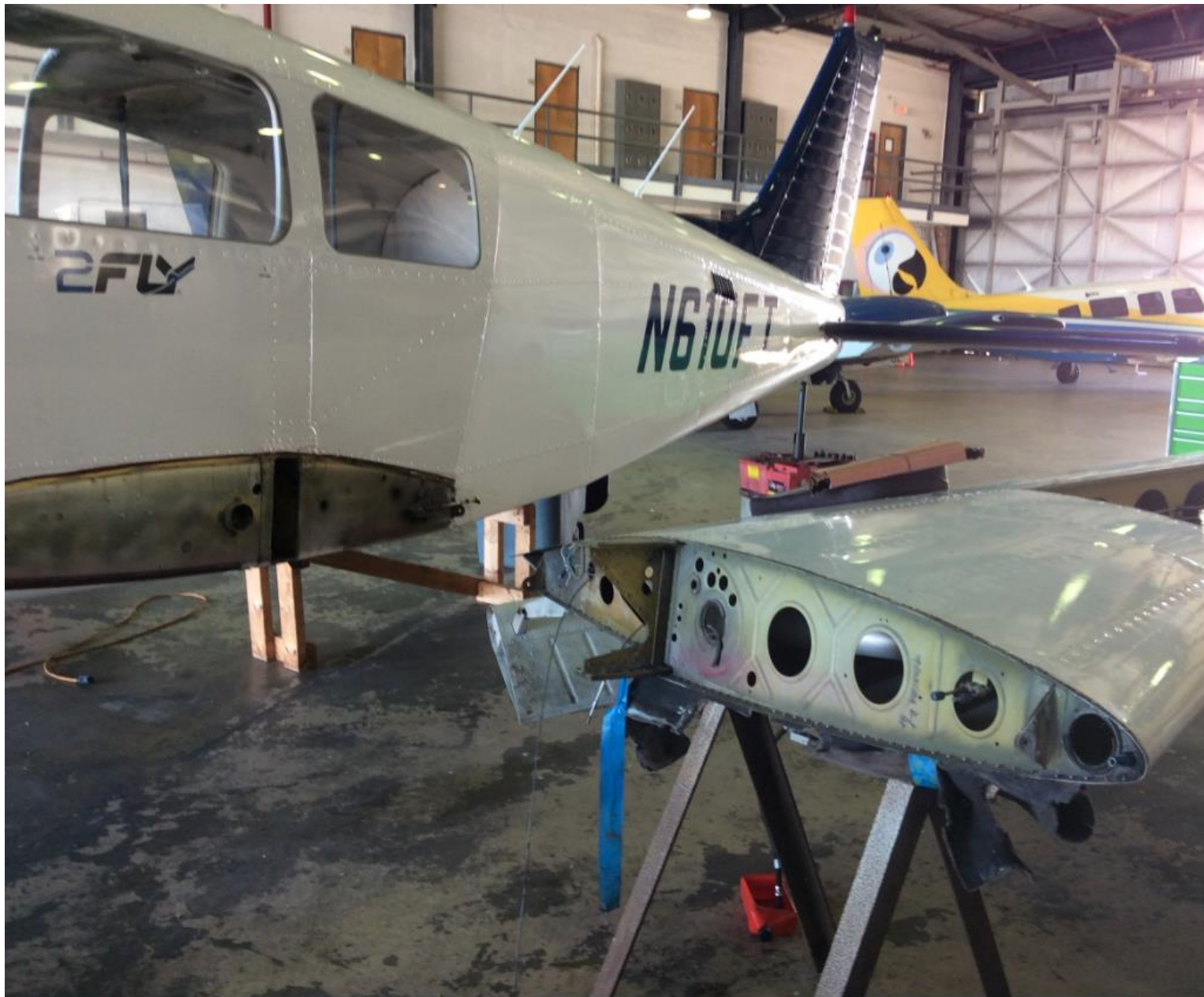
Photo 1 – View of damaged spar (Photo courtesy of the FAA)
