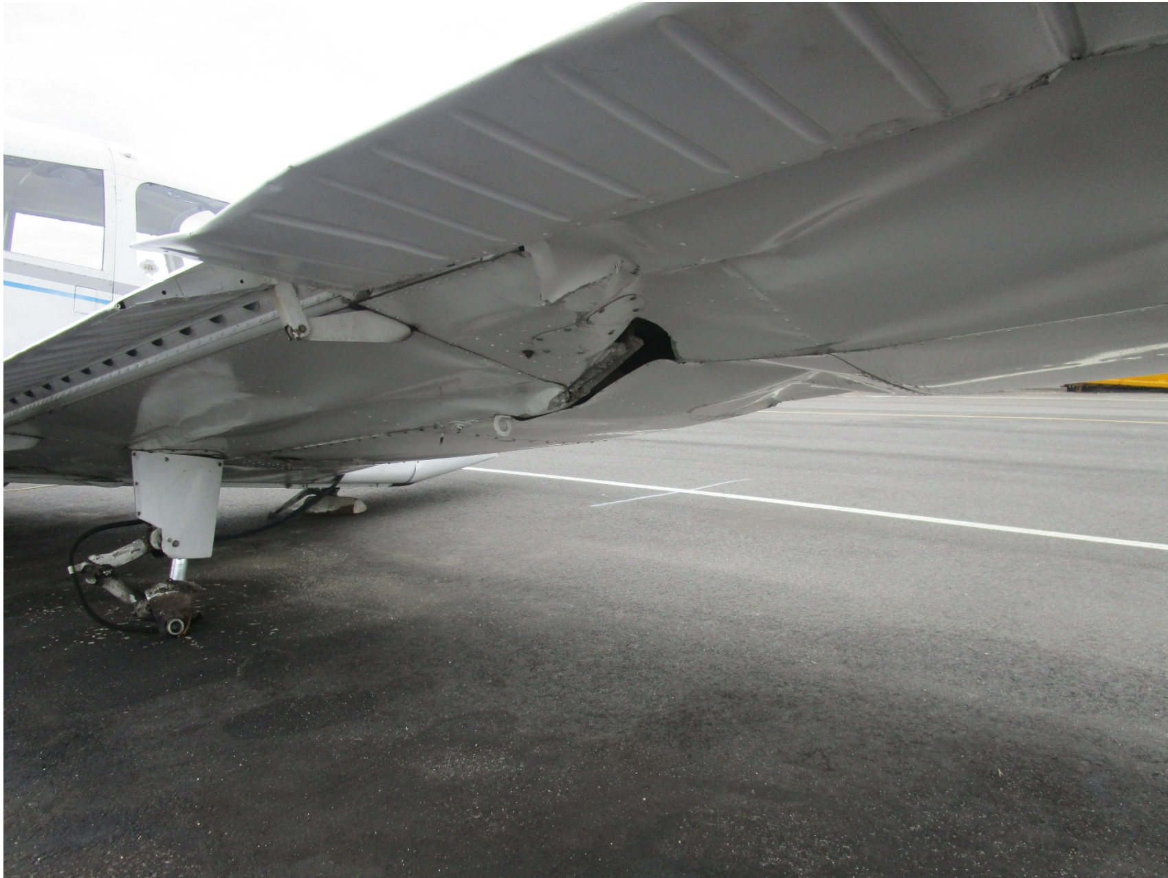
Photo 1 – View of right wing damage from underneath (Photo courtesy of the FAA)
