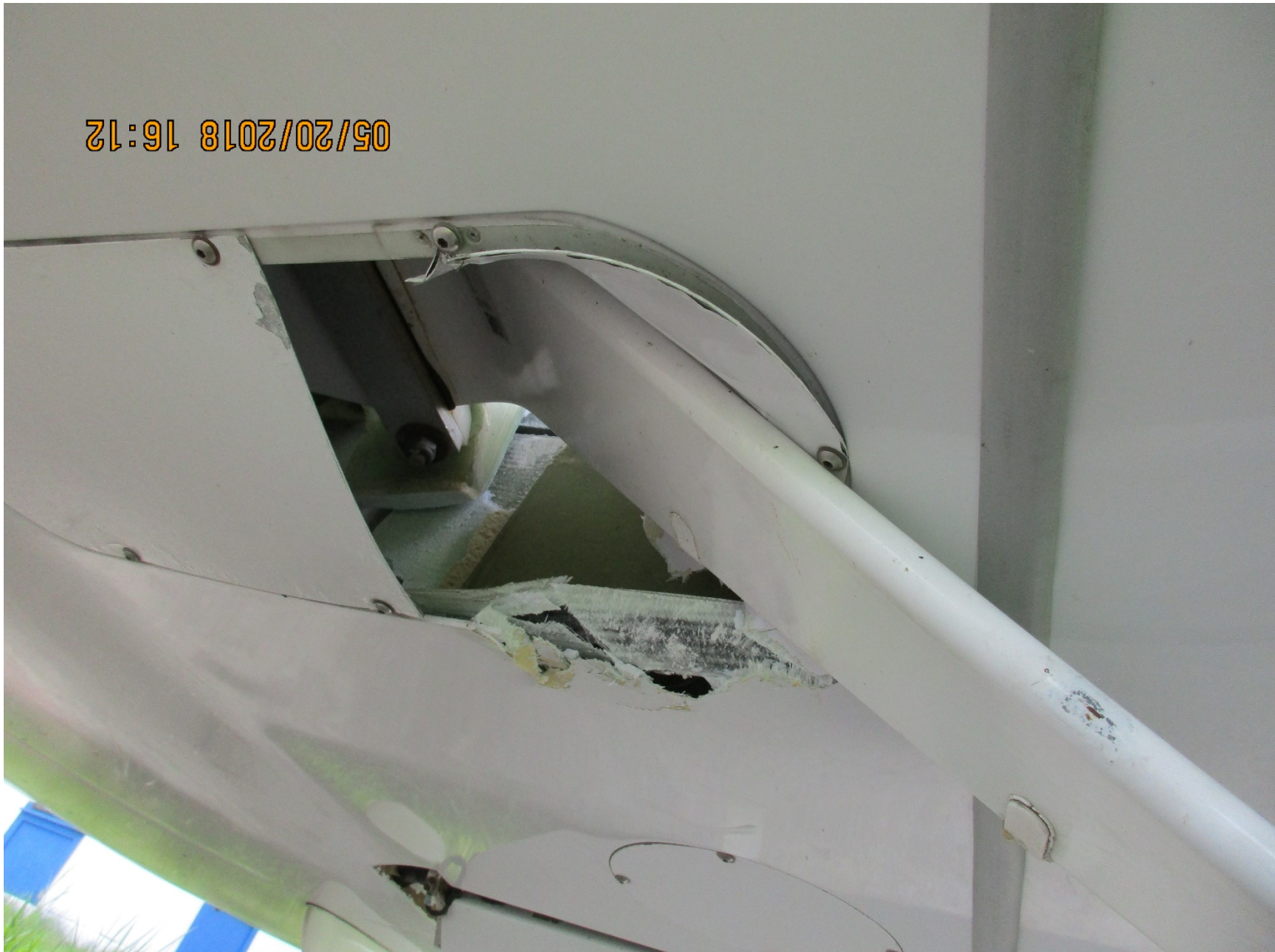
Photo 2 – View of damaged left wing from underneath (Photo courtesy of the FAA)
